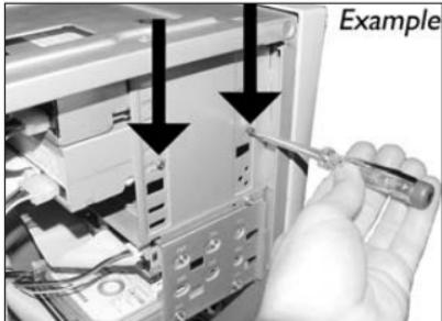
**EN** Secure the drive with the screws (if possible on both sides).
