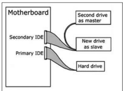
**EN** If you add a drive, check the drive has which remains in the PC ("Master" or "Slave", see step 11), remember the OTHER setting.
