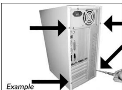
**EN** Put the screws (if there were any) back in and reconnect the cables.
