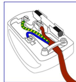
Before replacing the plug cover, make certain that the cord grip is clamped over the sheath of the lead - not simply over the three wires.
