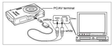
By using the AV cable, you can take pictures and play back captured images on equipment with a video IN jack, such as a TV. Make sure the camera and TV are turned off before connecting the camera to the TV.
