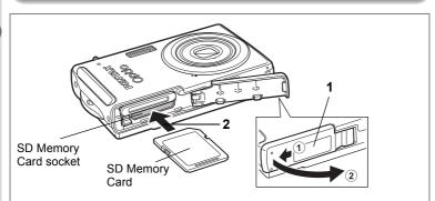
This camera uses either an SD Memory Card or an SDHC Memory Card. (Both cards are referred to as SD Memory Cards hereafter.) Captured images and sound files are saved on the SD Memory Card if a card is inserted in the camera. They are saved in the built-in memory if a card is not inserted. (p.32)
