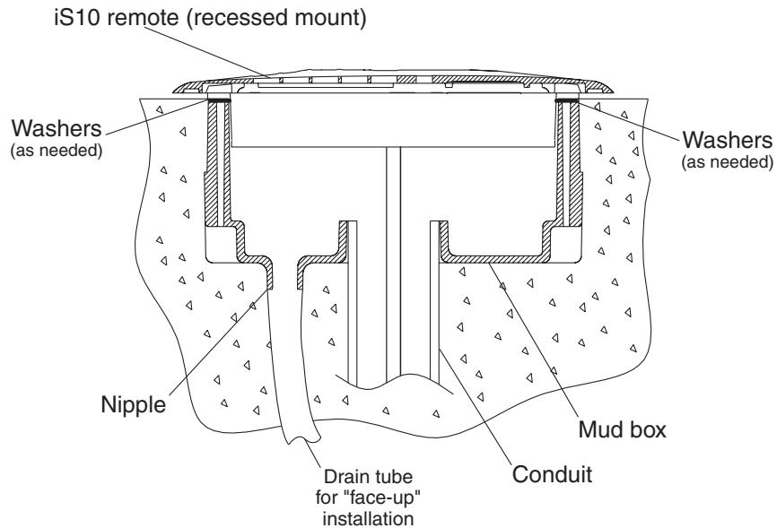
A nipple has been added to the mud-box for drainage if necessary. Cut the end of the nipple and attach a piece of  $\frac{1}{2}$  in. tubing. Run the tubing to appropriate drainage location away from the remote before finishing the deck or spa wall.
