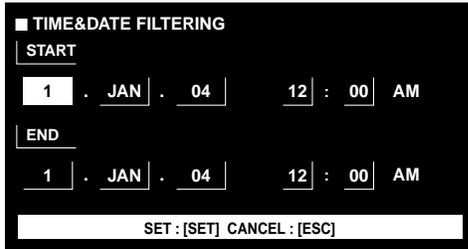
Move the cursor using the arrows button and rotate the jog dial to enter the time and date.
