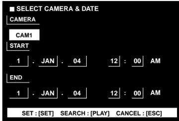
The VMD search window will be displayed. Enter a camera channel number and time range on the VMD search window for the VMD search. To search using the same conditions as the previous search, press the PLAY/PAUSE button. Go to step 13 when the VMD search is performed and a list of the results is displayed after the PLAY/PAUSE button is pressed.
