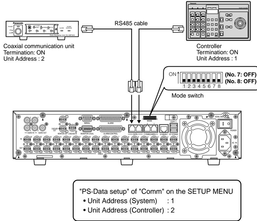
● When connecting this unit with a system device
