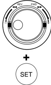
Press the SET button while holding the rotated shuttle ring to hold a desired playback speed. (Playback speed will be held even though the shuttle ring is released.)
