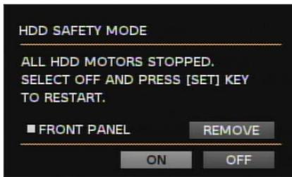
Move the cursor to OFF using the arrows button and press the SET button.
