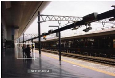
Press the SET button to determine the selected point as the end point of the motion detection area.
