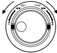
Rotating the shuttle ring will change the playback speed (1/2x, 1x, 2x, 5x, 10x, 20x) according to rotated degree. When the shuttle ring is held in the 20x position (rotated to the end) for 5 seconds, the playback speed will be 50x. When the shuttle ring is held 5 more seconds after the playback speed became 50x, the playback speed will be 100x.
