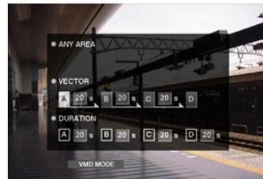
2 Set the detection mode. Move the cursor to the desired detection mode using the arrows button (▼ ▲ ◀ ▶). Move the cursor on the desired detection mode using the arrows button (◀ ▶) and check the radio button next to the selected mode using the jog dial. Refer to the following for further information about each of the detection modes.
