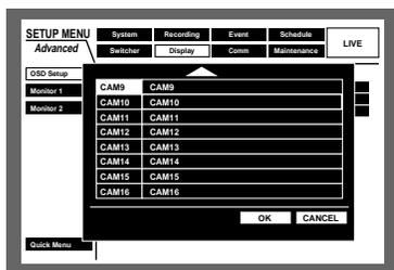
5. Press the arrows button (▼ ▲ ◀ ▶) to move the cursor to "OK" and press the SET button. When the arrows button (▼) is pressed while "OK" or "CANCEL" is selected, the camera title pop-up window for CAM9 - 16 will be displayed. Repeat steps 2 - 4 to enter the camera title for CAM9 - 16.
