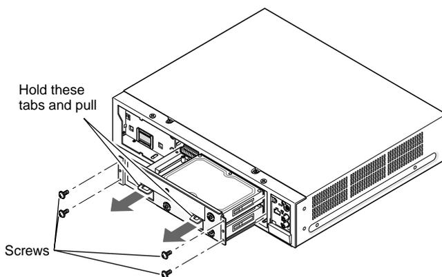
Only the upper and lower holes on both sides will be used when fixing by screws even though there are 3 holes each on both sides.
