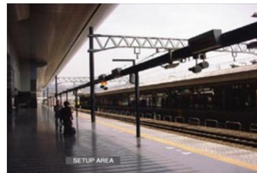
Press the SET button to determine the selected point as the start point of the motion detection area.
