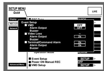
**2** Move the cursor to the item to be set using the arrows button (▼ ▲), and rotate the jog dial to select the parameter.
