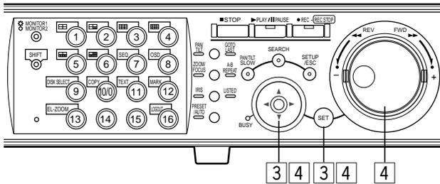
**3 Perform the settings for data copy (camera channel, time range, the disk on which images are to be copied). Move the cursor to each setting item using the arrows button and select a parameter by rotating the jog dial. (It is possible to change only the CAMERA parameter settings by pressing the SET button.)**
