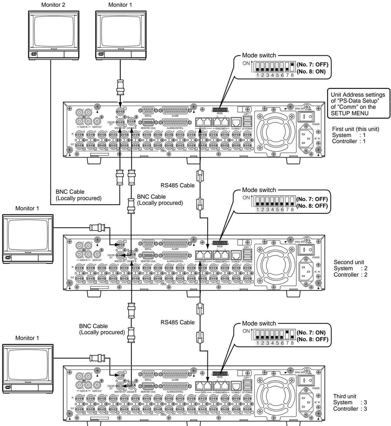
● When the PS-Data compatible device is connected to the first unit
