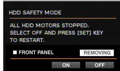
Detach the cable from the front panel and start replacing the built-in hard disk.
