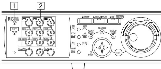
**1 Press the MONITOR1/MONITOR2 button to select the monitor.**
