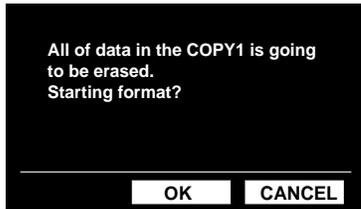
**8 Move the cursor to "OK" using the arrows button and press the SET button to start formatting.**
