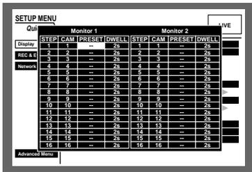
**5** Rotate the jog dial to select a preset position number for which image is displayed in "STEP 1" from the following.
