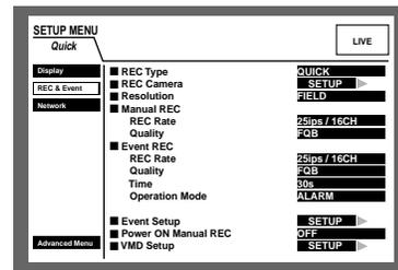
**1** Move the cursor to "Event Setup" using the arrows button (▼ ▲) and press the SET button.
