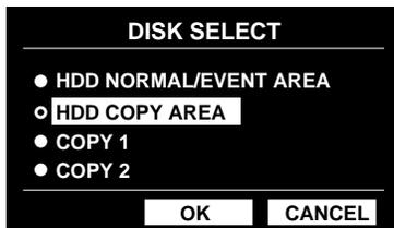
When "HDD NORMAL/EVENT AREA" or "HDD COPY AREA" is selected, the recording event list window will be displayed. (Refer to page 29 for further information about the recording event list window.)
