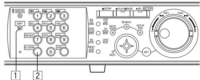
**1 Press the SHIFT button when monitoring live images on a single screen.**
