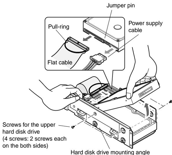
5. Detach the flat cable and the power supply cable from the hard disk drive. Detach the flat cable only from the hard disk drive. (Do not detach the flat cable from the circuit board.)
