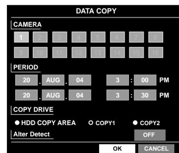
The DATA COPY window will be displayed on monitor 2 and the VGA monitor.
