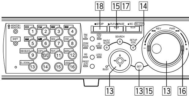
**13** Move the cursor to select a detection mode using the arrow buttons and rotate the jog dial to check the radio button next to the selected detection mode. Press the SET button to determine the selection.
