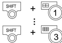
It is possible to display recorded images in multi-screen format (4/7/9/10/13/16 for the WJ-HD316A, 4/7/9 for the WJ-HD309A).
