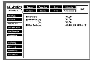
● **[Disk End Mode] Set actions to be taken when the available hard disk space has run out**
