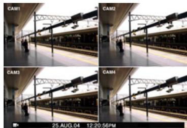
When monitor 2 is selected in step 1, live images will also be displayed on the selected multi-screen on the VGA monitor.
