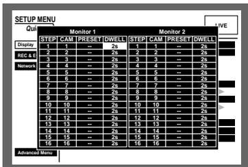
**7** Rotate the jog dial to select an interval time to go to the next sequential step from 1 - 30 seconds (in 1 second intervals).
