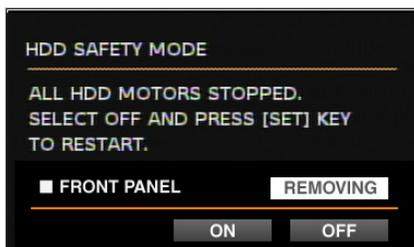
Detach the cable from the front panel and start replacing the built-in hard disk.
