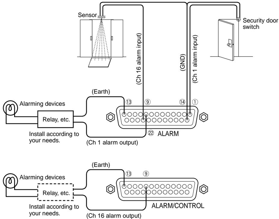
Time and polarities of the ALARM/CONTROL terminal and the ALARM terminal
