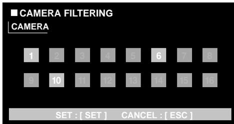
Select camera channel numbers (1 - 16 for the WJ-HD316A, 1 - 9 for the WJ-HD309A) using the arrows button to move the cursor, and rotate the jog dial to apply filtering. It is possible to select camera channels using the camera selection buttons [1] - [16] for the WJ-HD316A ([1] - [9] for the WJ-HD309A).
