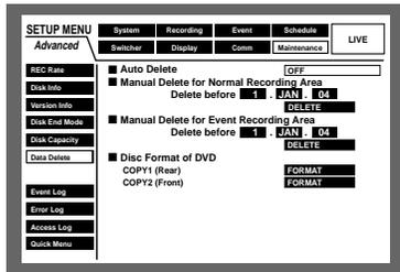
**6 Move the cursor to "Manual Delete for Normal Recording Area" or "Manual Delete for Event Recording Area" using the arrows button, and set time and date using the jog dial.**
