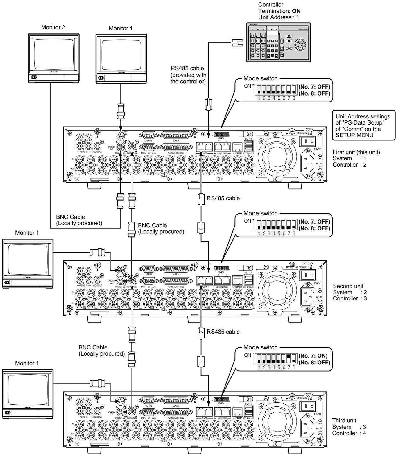
● When the PS-Data compatible device is connected to the third unit
