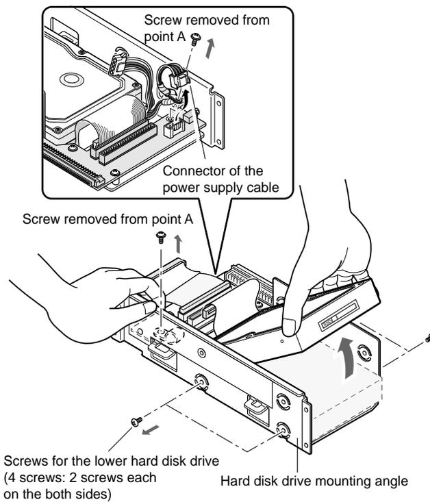
6. Install the new hard disk drive in the reverse order used for detaching the hard disk drive.
