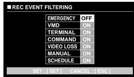
Move the cursor to select the recording event (refer to page 29) using the arrows button (▼ ▲) and rotate the jog dial to ON.
