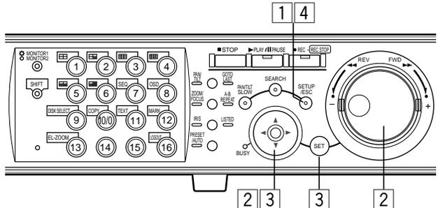
**1 Press the SETUP/ESC button for 2 seconds or more.**
