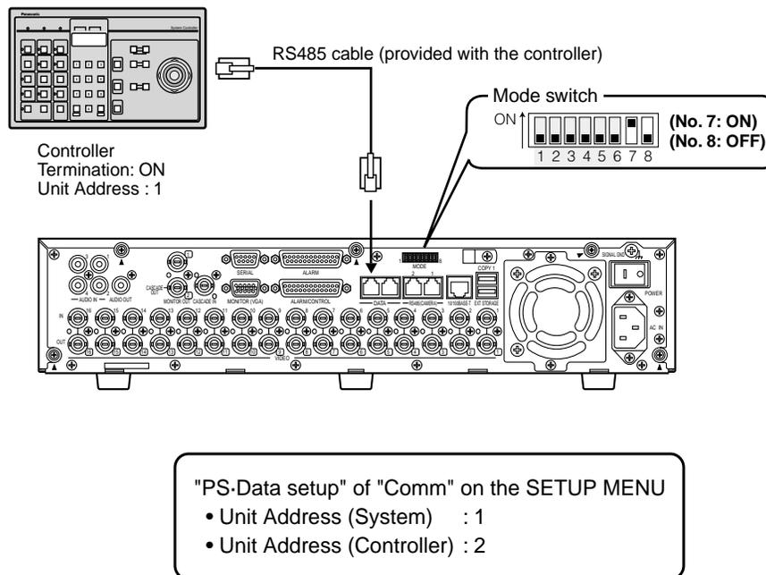
● When installing this unit between a controller and a system device
