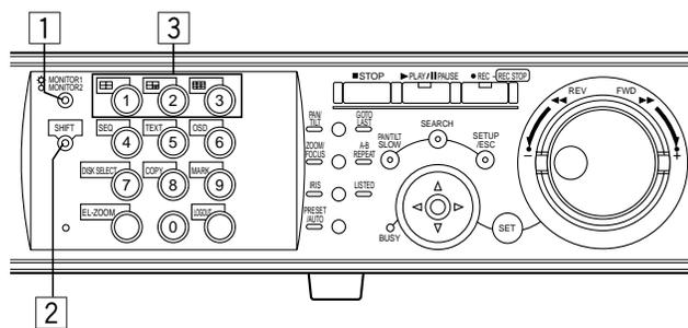
**1 Press the MONITOR1/MONITOR2 button to select the monitor.**
