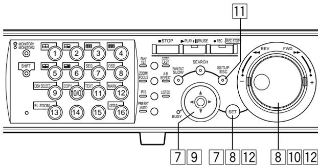
**7** Move the cross cursor using the arrows button to a point to be determined as the end point of the motion detection area.
