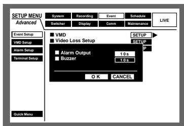
The following are available for the alarm output duration. When OFF is selected, the alarm output will not be supplied.
