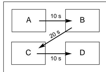
Motion is detected in area B within 10 seconds after being detected in area A.
