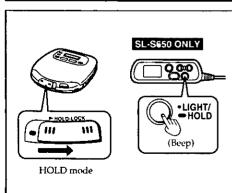
This function causes the unit to ignore short, accidental button presses. (When the unit is in HOLD status, the cover will not open even when the OPFN button is pressed.)
