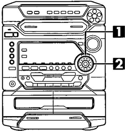
It is possible to use the acoustic image equalizer (AI EQ) together with the surround effect to create your own sound effect. The AI EQ equalizer uses the SOFT, SHARP, HEAVY and LIGHT sound quality coordinates to achieve subtle sound quality settings with ease.
