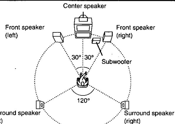
The front, center, and surround speakers should be placed at approximately the same distance from the seating area. The angles in the diagram are approximate.
