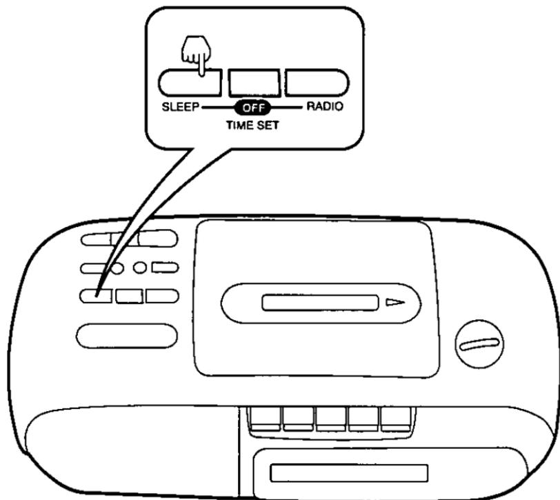
You can set the clock radio to play up to about 59 minutes, the shut off automatically.
