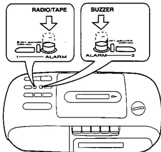
The buzzer alarm and the radio (or tape alarm) are set at the same time. Both alarms will activate simultaneously.
