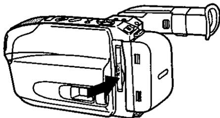
To remove, press in on the Remote as shown by the arrow and it will release.
