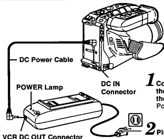
**1** Connect the VCR DC OUT on the AC Adaptor to the DC IN on the Palmcorder with the DC Power Cable (supplied).
