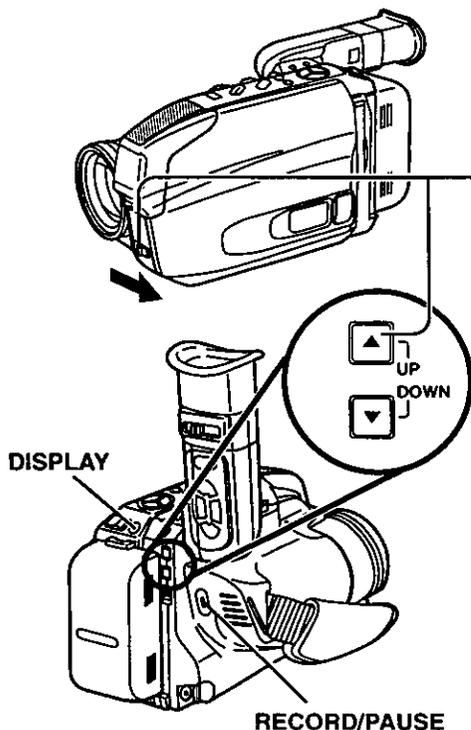
**1** While pressing the UP ▲ button, set the POWER switch to CAMERA.
