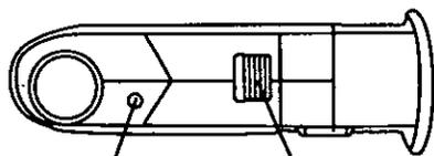
**\*Note:** These controls have been set at the factory. It is not necessary to adjust these controls under normal circumstances. But, should it become necessary, be careful to make the adjustment with a small, slender screwdriver so as not to damage the miniature control.
