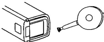
**3** Remove any lint or dust particles with a blower, available at photography stores. Do not touch lenses with fingers. Now, replace the eyepiece.
