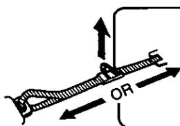
**1** Pull a loop of the strap loose from the buckle.
