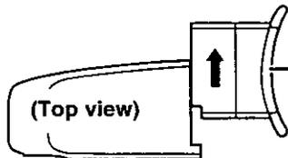
**2** Remove the eyepiece. (Do not twist.)
