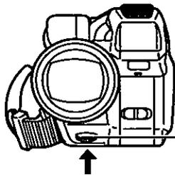
For Auto Focus mode, it may be necessary to **press MANUAL FOCUS**, so that "MF" does not appear in the EVF.
