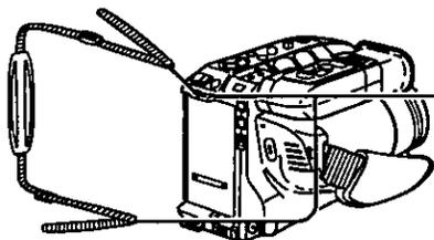
**2** Thread the strap ends through the Strap Attachment Rings.
