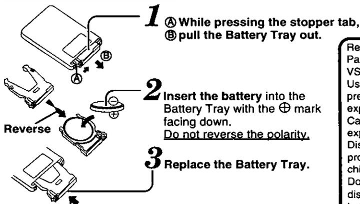
Replace battery with Panasonic PART NO. VSBW0004 (CR2025) only. Use of another battery may present a risk of fire or explosion. Caution-battery may explode if mistreated. Dispose of used battery promptly. Keep away from children. Do not recharge, disassemble or dispose of in fire.
