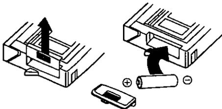
Remove the Battery Compartment lid and insert the AA size battery.
