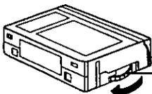
**1** Turn the Tape Wheel on the **VHS** cassette in the direction of the arrow to reduce any slack.
