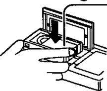
**3** Insert the **VHS** cassette with the window facing up and to the left. Then, snap the lid shut.
