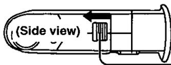
**1** Slide and hold the EYEPIECE RELEASE button.
