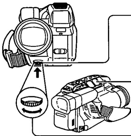
**1** Press **MANUAL FOCUS** so that "MF" (Manual Focus) appears in the EVF.
