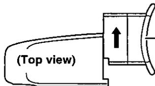
**2** Remove the eyepiece. (Do not twist.)
