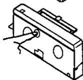
**2** Hold the PlayPak securely in one hand. Put your finger through the hole in the bottom of the PlayPak and push the cassette out.
