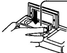
**3** Insert the **VHS** cassette with the window facing up and to the left. Then, snap the lid shut.
