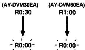
• It will take several seconds for the tape remaining indicator to operate after the tape starts moving.
