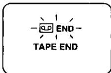
When the tape is about to end in REC mode, "□□ END" will flash and "TAPE END" will appear for 5 seconds.
