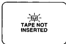
If the Palmcorder is in CAMERA mode without a cassette inserted, "□□" will flash and "TAPE NOT INSERTED" will appear for 5 seconds. Recording will not start.
