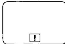
When the LCD monitor is rotated 180° so that it faces the same direction as the lens, the "!" mark indicates that a warning message exists. To view the warning, return the LCD monitor to the original position.
