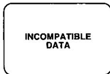
If you play a tape recorded in a format other than NTSC or you try to copy a copy-protected tape, "INCOMPATIBLE DATA" will continuously appear. This message also appears if REC is pressed when DV/Analog is input and the copy of copyrighted information is prohibited.
