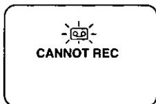
When Audio dub is performed and the sliding record tab is open, or a blank portion of tape is detected, "□□" will flash and "CANNOT REC" will appear for 5 seconds.
