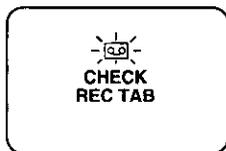
If the Palmcorder is in CAMERA mode with the cassette sliding record tab opened, "□□" will flash and "CHECK REC TAB" will appear for 5 seconds. Recording will not start.
