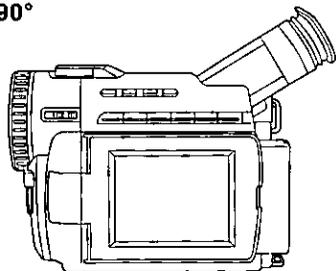
You can place the Palmcorder on a table, etc. for viewing. Rotate the LCD Monitor 180° and swing it up against the Palmcorder body as shown.
