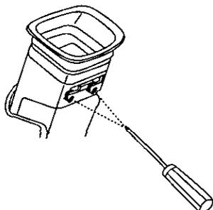
**6** Replace the EVF Eyepiece screws and tighten with a screwdriver.
