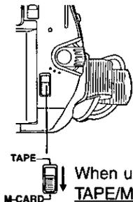
When using a MultiMediaCard, you must set **TAPE/M-CARD Switch** to **M-CARD**.
