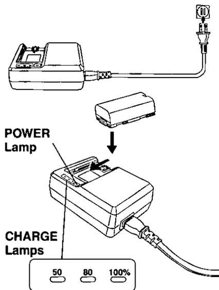
**1** Connect and plug in the Cable as shown.
