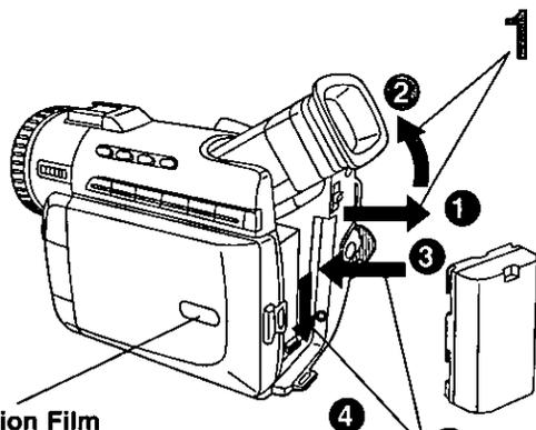
**1** Slide the Viewfinder backward to its fully expanded position and then tilt it upward.
