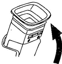
**1** Slide the Viewfinder backward to its fully expanded position and then tilt it upward.
