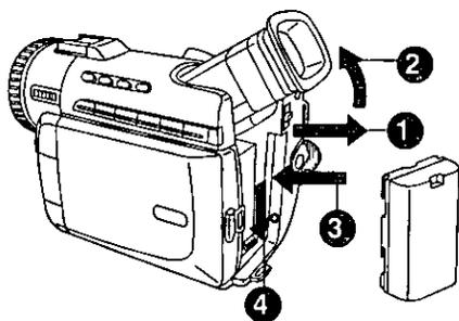
**1** Slide the Viewfinder backward to its fully extended position and then tilt it upward.
