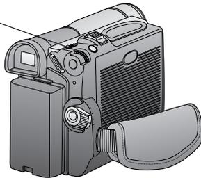
1 During Still mode, **rotate JOG KEY** to advance or reverse the picture one frame at a time.
