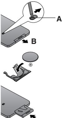
**1** Insert a slender pointed object, such as the tip of a ball-point pen into the slot so that it fits into the hole (as shown **A**). Then, while sliding to the right, pull the Battery Tray out with your fingernail.
