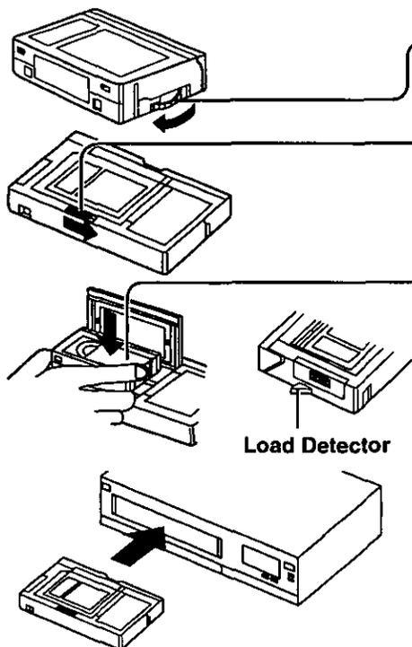
**1** Turn the Tape Wheel on the **VHS** cassette in the direction of the arrow to take up any slack.
