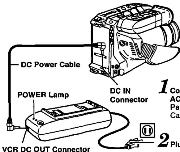
**1** Connect VCR DC OUT on the AC Adaptor to DC IN on the Palmcorder with the DC Power Cable (supplied).
