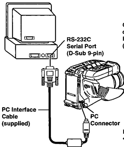
Connect the supplied PC connecting cable to the PC connection jack on the Palmcorder and a serial port on the PC (Personal Computer).
