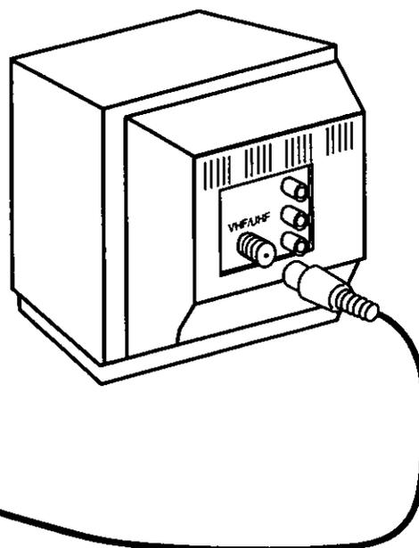
RF Coaxial Cable (VCR-TV Connection Cable) (supplied)
