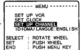
**2** Rotate and push the WHEEL to select SET UP CHANNEL.
