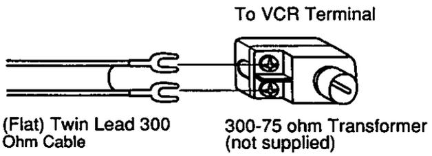
**Case 2: Twin Lead & Coaxial Cables**
