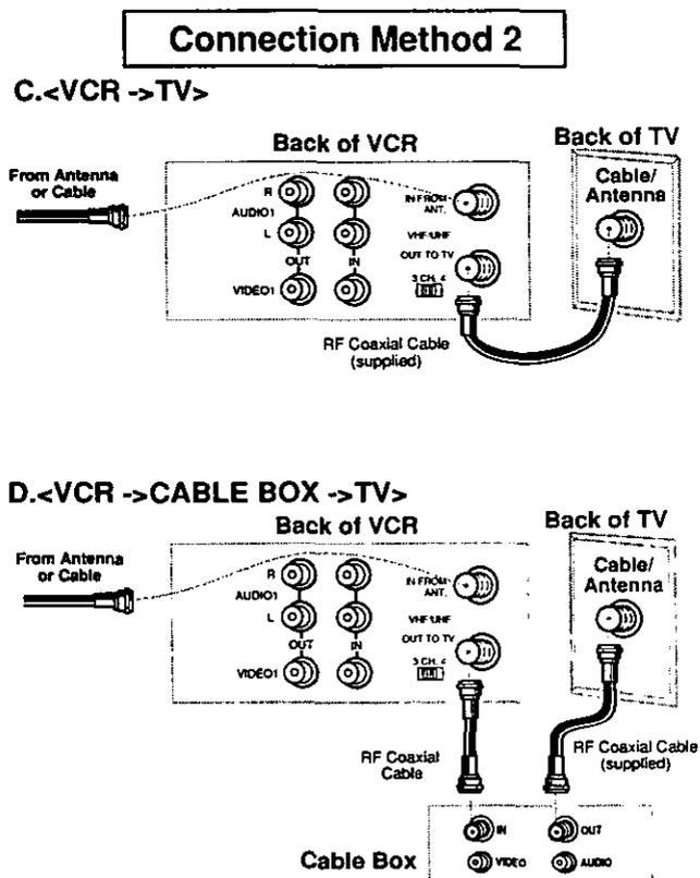
Back of models PV-4655S and PV-4665S VCR are shown here.
