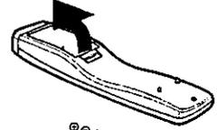
**2** Install three batteries as indicated inside the Battery Compartment.
