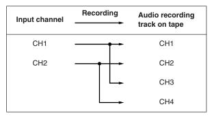
■ Serial digital multiplex signal input (SDI: option) (Setup menu item No.712 setting: CH1/CH2)
