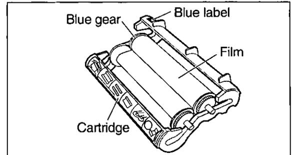
**9** Lock the four gears of the film by (A) pushing back the top side gears and (B) pulling the bottom side gears forward until they lock into place.
