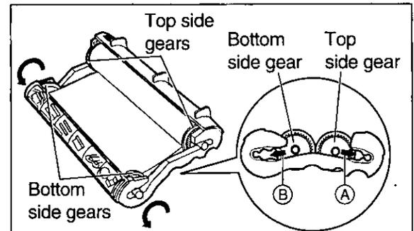
**10** Insert the film cartridge by matching the blue label on the cartridge with the one on the unit.
