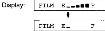
When the film indicator points to this position, the remaining film will print up to 25 pages of letter size documents. Prepare a new film or film cartridge for replacement.
