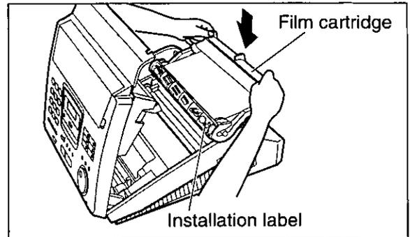
**7** Make sure that the blue label on the cartridge matches the one on the unit.
