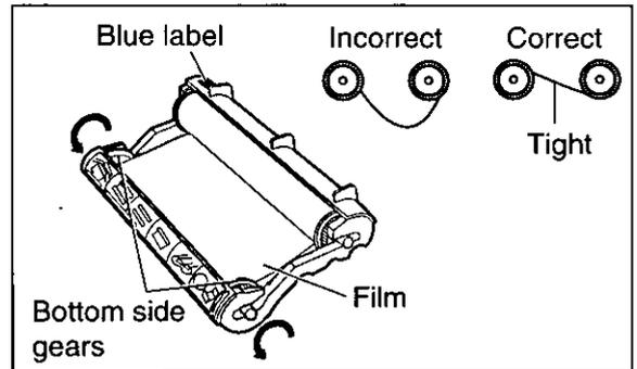
**6** Install the film cartridge into the unit.
