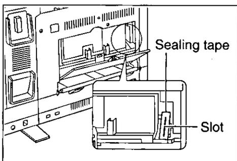
Put and fix the sealing tape to close the slot on the rear side of the toner cartridge if you have not covered the slot.
