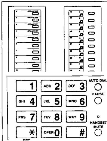
Enter the desired phone number by using the direct call station key, the speed dial station, or a full number.
