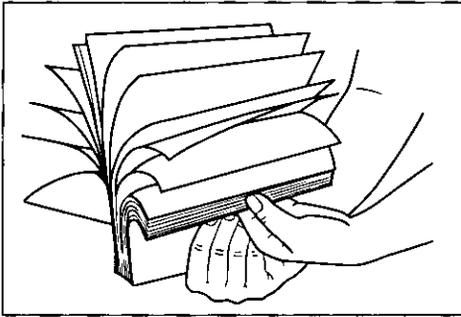
Fan the stack of paper to avoid a paper jam.
