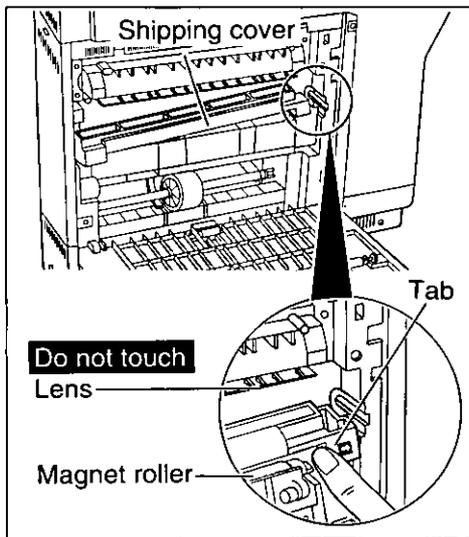
Press the tab of the shipping cover firmly toward the front, and lift the rear side of the shipping cover up and remove it by pulling it outward.
