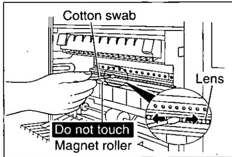
Wipe the lens by sliding the cotton swab from end to end 4 to 5 times.
