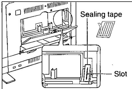
Remove the sealing tape from the storage bag provided. Peel one piece of tape from the paper backing and press it over the slot on the toner cartridge.
