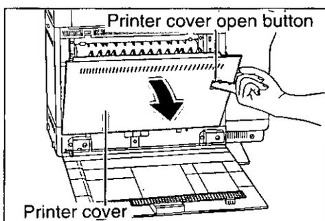
Open the printer cover by pulling the printer cover open button.
