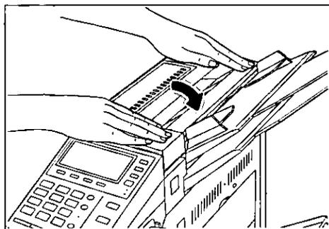
Close the upper cover carefully by pushing down until the cover locks into position.
