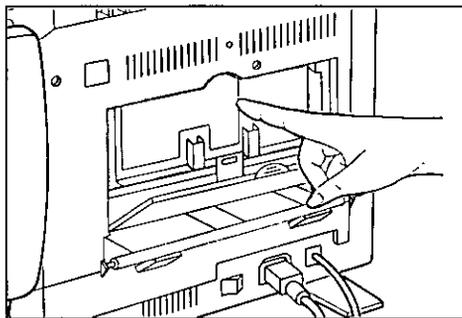
Tap the toner cartridge lightly to empty toner into the developer unit.
