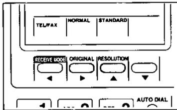
Set the contrast or resolution mode by using **ORIGINAL** or **RESOLUTION** if needed.
