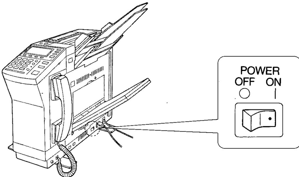
When turning the unit on, the display shows the following message for a while. After warming up, your unit will be ready to use.
