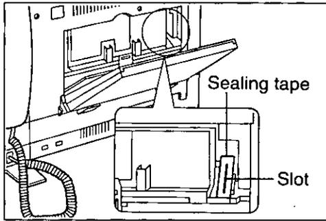
Peel one piece of sealing tape from the paper backing and press it over the slot on the toner cartridge.
