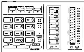
Enter the desired phone number by using the direct call station key, the speed dial station, or a full number.
