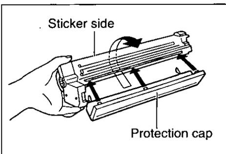
Replace the drum protection cap on the drum unit.
