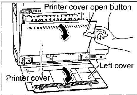
Open the left cover, and open the printer cover by pulling the printer cover open button.
