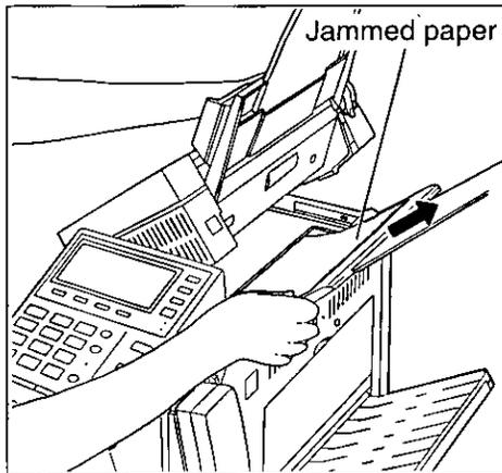
Remove the jammed paper by carefully pulling it up.
