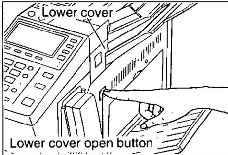
Push the lower cover open button, and open the lower cover completely until it clicks.
