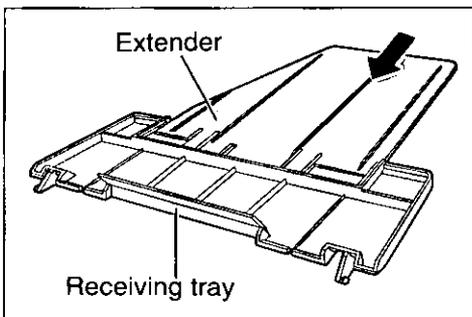
Insert the extender into the receiving tray.
