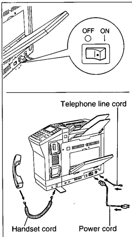
Turn the power off, then disconnect the power cord, telephone line cord, and handset cord.
