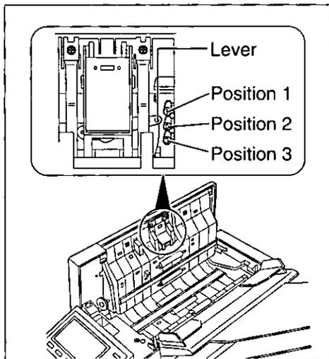
Shift the position of the lever on the document feeder unit by using an instrument with a pointed end, like a clip or ball-point pen.
