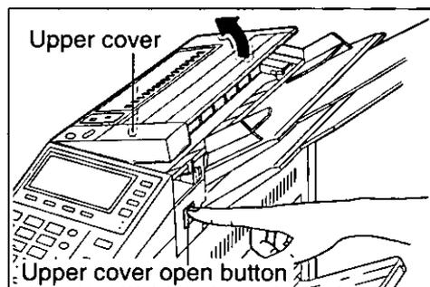
Open the upper cover by pushing the upper cover open button.
