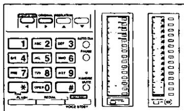
Enter the name associated with the speed dial station by using the dial keypad and the direct call station keys as character keys, and the cursor key (◀ or ▶).
