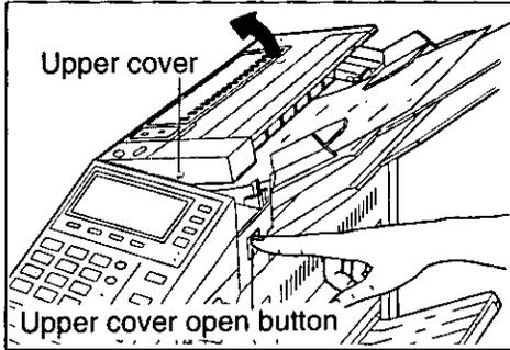
Open the upper cover by pushing the upper cover open button.
