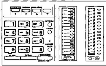
Enter the station name by using the dial keypad and the direct call station keys as character keys, and the cursor key ( ◀ or ▶ ).
