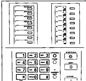
Enter the desired phone number by using the direct call station key, the speed dial station, or a full number.
