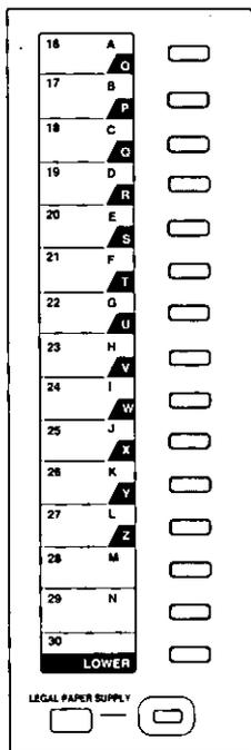
Open the station key cover. You can select the desired index by pressing the direct call station key that is corresponding to the index.
