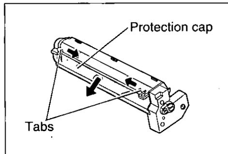
Remove the drum protection cap by pushing the right and left tabs inward.
