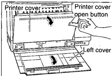
Open the left cover, and open the printer cover by pulling the printer cover open button.
