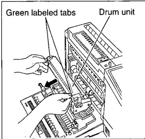
Remove the drum unit by slightly raising both green labeled tabs and pulling the drum unit outward.
