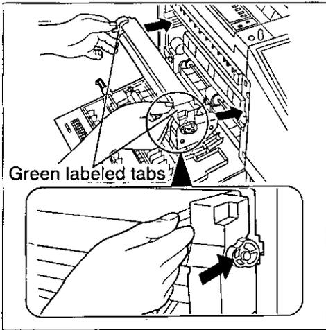
Install the drum unit by holding the green labeled tabs and pushing it firmly into place.
