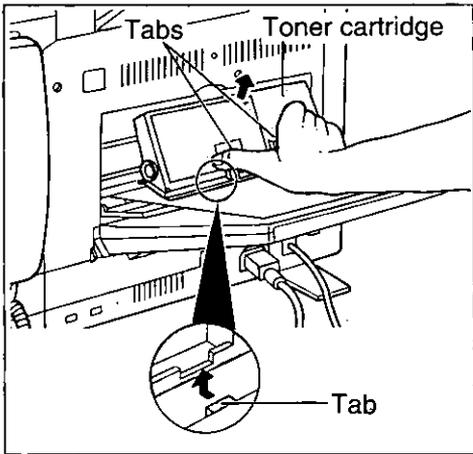
Remove the toner cartridge carefully by pushing both tabs firmly and raising it slightly.
