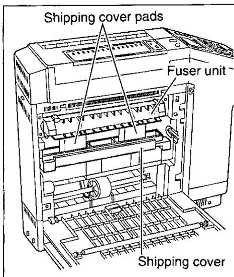
Install the shipping cover pads straight between the shipping cover and the fuser unit.
