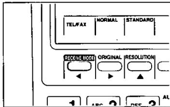
Press **RECEIVE MODE** to select the desired receiving mode.
