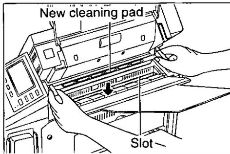
Insert the new cleaning pad into the slot by holding both side tabs.
