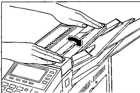
Close the upper cover carefully by pushing down until the cover locks into position.
