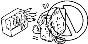
Keep the unit away from electrical noise-generating devices, such as fluorescent lamps and motors.
