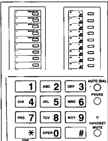
Enter the desired phone number by using the direct call station key or the speed dial station.
