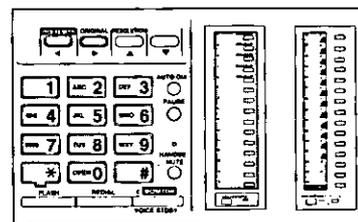
Enter the name associated with the direct call station by using the dial keypad and the direct call station keys as character keys, and the cursor key (◀ or ▶).
