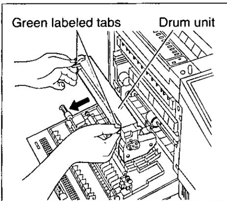
Remove the drum unit by slightly raising both green labeled tabs and pulling the drum unit outward.
