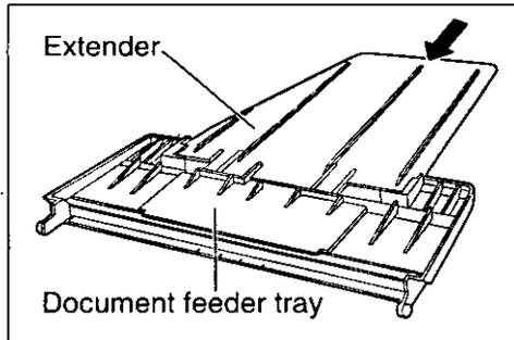
Insert the extender into the document feeder tray.
