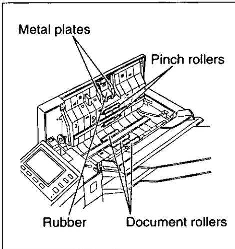
Clean the document rollers, pinch rollers, and rubber with a cloth moistened with isopropyl rubbing alcohol, then dry thoroughly to prevent paper from jamming.
