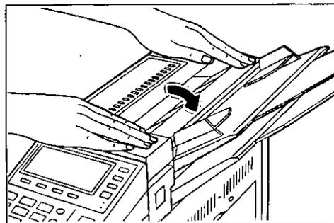
Close the lower cover carefully by pushing down until the cover locks into position.
