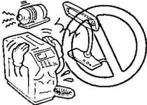
The unit should be kept free from dust, moisture, high temperature, and vibration.
