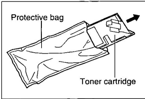
Open the protective bag and remove the toner cartridge.
