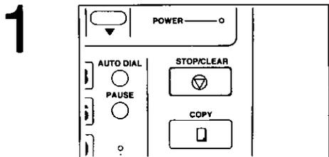
Press **STOP/CLEAR** twice after setting the multistation transmission.
