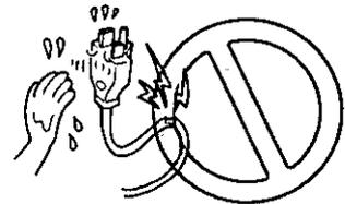
Keep the unit dry. Never operate the unit if liquid has been spilled into it. Immediately unplug the unit, have it inspected by service technician. Fire and shock hazards can result from electrical shorts caused by liquid contact inside.
