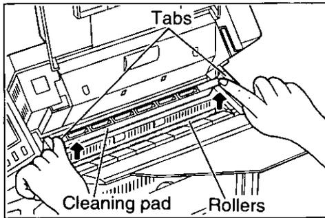
Remove the cleaning pad by lifting both tabs up.
