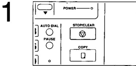
Press **STOP/CLEAR** after setting the delayed transmission.
