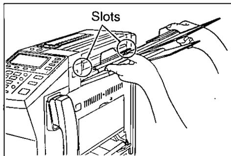
Insert the pins of the document feeder tray firmly into the slots on both sides of the unit, and the document feeder tray locks into position.
