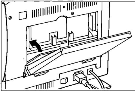
Remove the sheet from the cartridge compartment cover, and close the cover.
