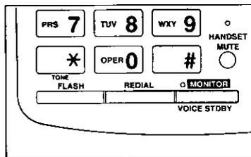
After pressing **MONITOR** or lifting the handset, press **REDIAL**.
