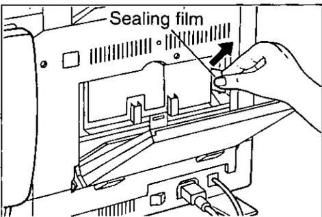
Grasp the sealing film. While holding the unit with your other hand, firmly pull the film from the cartridge.
