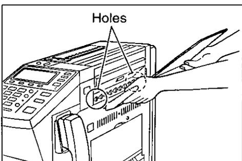
Insert the pins on the receiving tray firmly into the holes on both sides of the unit.
