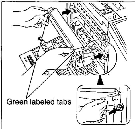
Install the new drum unit by holding the green labeled tabs and pushing it firmly into place.
