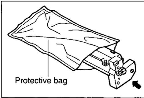
Pack the drum unit into the protective bag.
