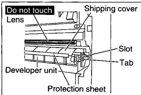
Press the right side of the shipping cover firmly, and insert the tab of the developer unit into the slot until it clicks into place.
