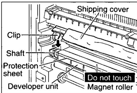
Hook the left clip of the shipping cover on the shaft of the developer unit, and press the clip firmly.
