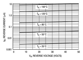
Figure 3. Leakage Current
