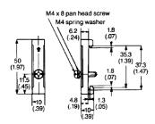
Note: Use of Type PFP-M end plate is recommended to secure the socket on the mounting track. Be sure that the engraved arrow mark on the surface of the end plate faces upward and then tighten the screw firmly with a screwdriver.
