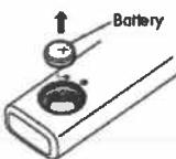
3. Insert the new battery with the "+" pole facing up as shown in the diagram.
