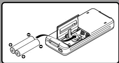
Insert the batteries in the direction inscribed on the inside of the recorder's battery compartment. In addition, when inserting the batteries, insert them so that the tape is under the batteries, as shown in the illustration. The batteries can then be removed easily by pulling up the tape. **When pulling on the tape the batteries may suddenly pop out, so be sure to press down lightly on the batteries with your finger while pulling.**
