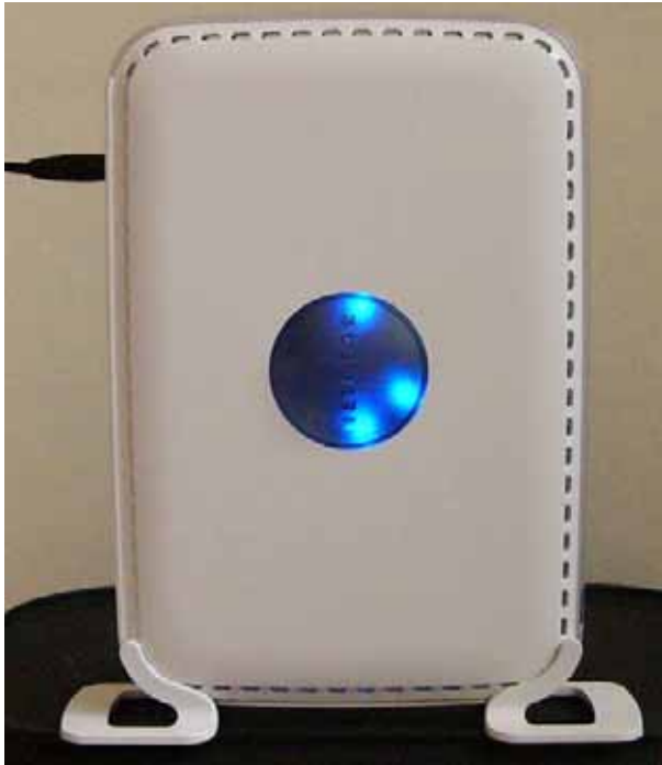
Figure 4-1: Vertical orientation required on metallic surfaces
