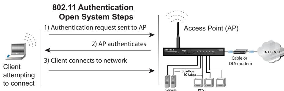
**Figure 4-1: 802.11 open system authentication**
