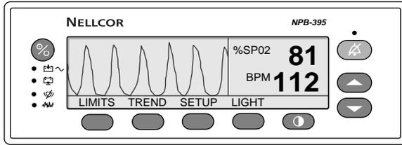
**Figure 16: Monitoring Mode Display - PLETH View**
