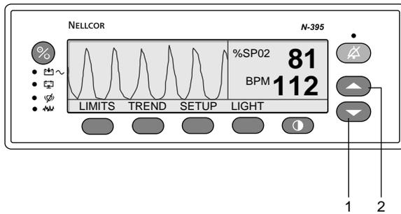
**Figure 18: ADJUST UP and ADJUST DOWN Buttons**
