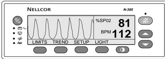
**Figure 19: Monitoring Mode Display - PLETH View**
