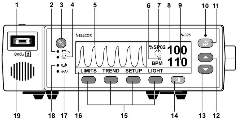
**Figure 7: N-395 Front Panel - PLETH View**
