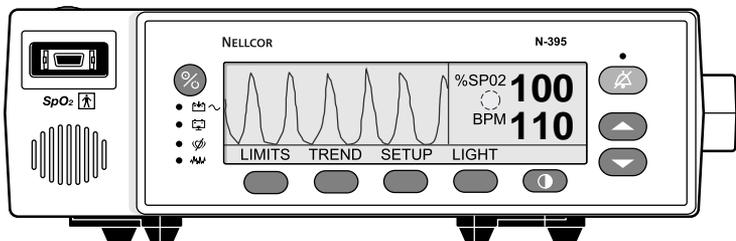
**Figure 2: Front Panel with PLETH View Displayed**
