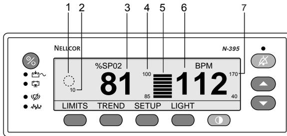
**Figure 8: N-395 Front Panel - BLIP View**
