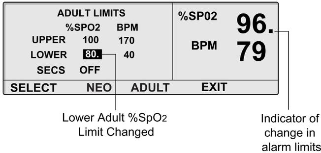
**Figure 31: %SpO<sub>2</sub> Alarm Limits Changed**
