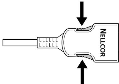
**Figure 4: Disconnecting Cable from Monitor**
