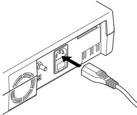
**Figure 11: Connecting the Power Cord to the Monitor**
