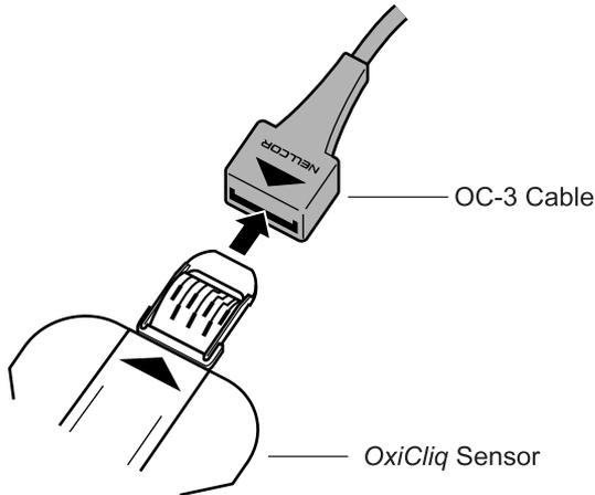
**Figure 14: *OxiCliq* Sensor and OC-3 Sensor Cable Connection**
