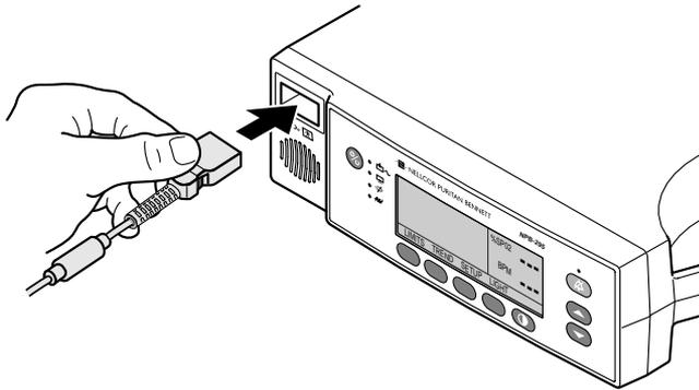
**Figure 15: Connecting a Sensor to the Monitor**
