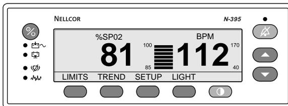
**Figure 20: Monitoring Mode Display - BLIP View**
