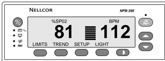
**Figure 17: Monitoring Mode Display - BLIP View**
