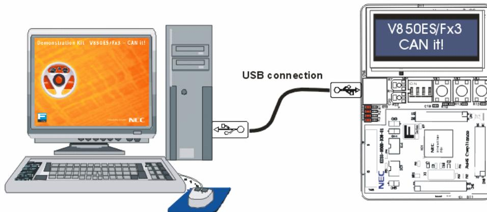
Figure 1: V850ES/Fx3 – CAN it! system configuration
