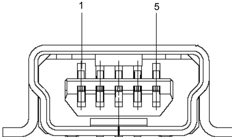
Figure 3: Connector CN6, USB Mini-B Type Host Connector Pin Configuration
