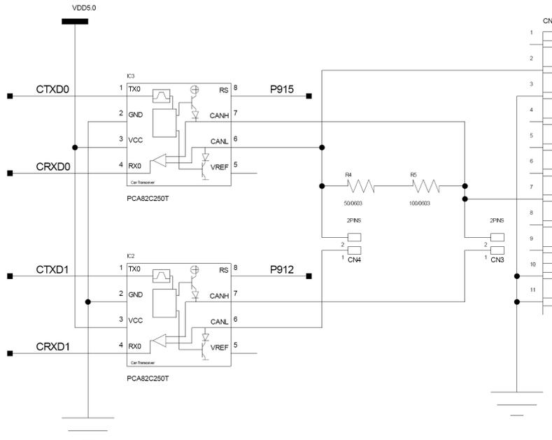
**Figure 5: CAN transceivers**
