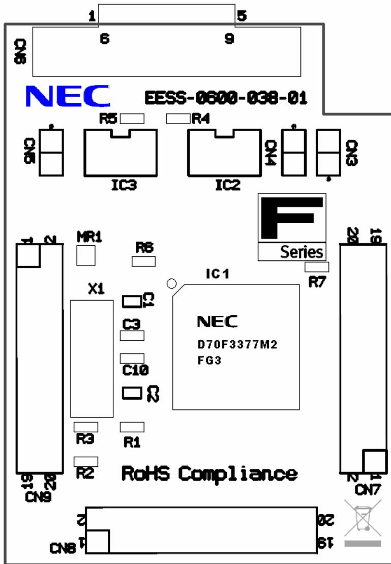
Figure 4: V850ES/Fx3 – CAN it! CPU module components
