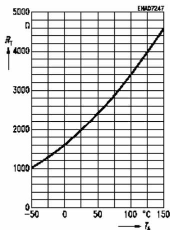
The temperature at the sensor can be calculated from the change in the sensors resistance from the following equation, which approximates the characteristic curve:
