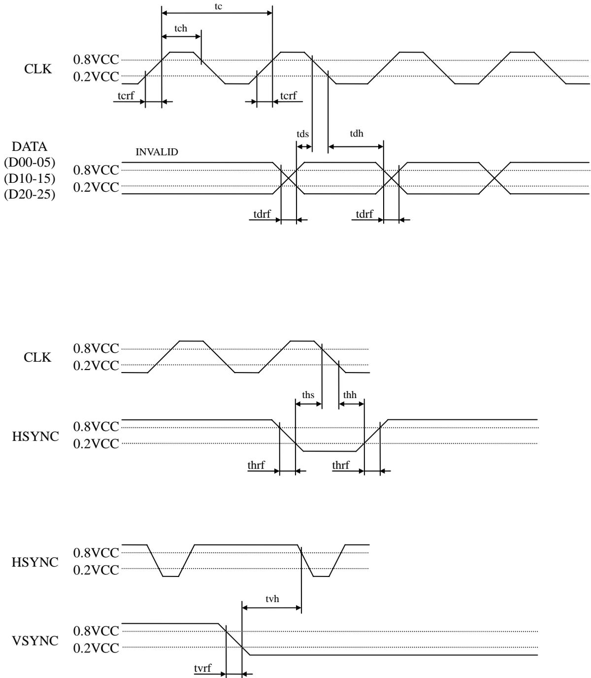
Note1: Unless otherwise specified, the input level is defined to be  $V_{IH} = 0.8V_{CC}$ ,  $V_{IL} = 0.2V_{CC}$ .
