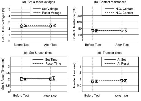
Figure 5.6 (4) Shock Test
