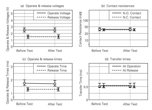
Figure 5.8 (1) Resistance to Reflow Solder Heat
