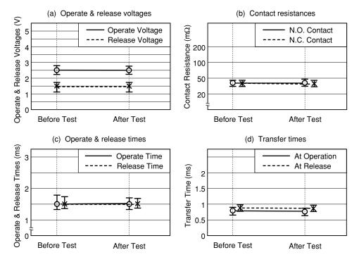
Figure 5.6 (1) Shock Test
