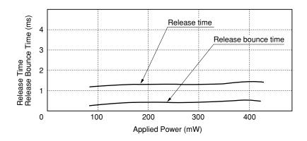
Figure 3.5 Driving Power vs. Timing
