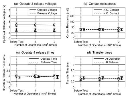
Figure 5.19 Resistive Load Test G
