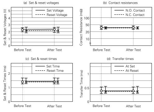
Figure 5.8 (2) Resistance to Reflow Solder Heat
