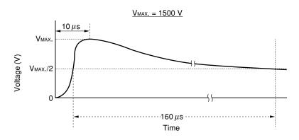
Figure 3.10 Surge Voltage Waveform
