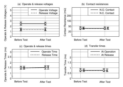
Figure 5.7 (1) Resistance to Solder Heat Test
