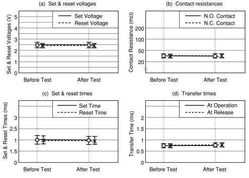
Figure 5.4 (4) Heat Shock Test
