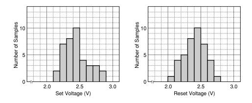
Figure 4.1 Operate & Release Voltages
