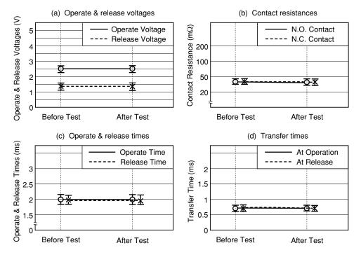
Figure 5.4 (1) Heat Shock Test
