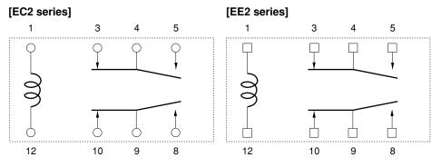
Internal Connection of Relay (Bottom View)
