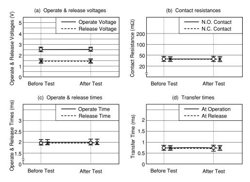
Figure 5.2 (3) Low-temperature Test
