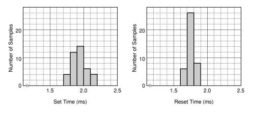
Figure 4.2 Operate & Release Times
