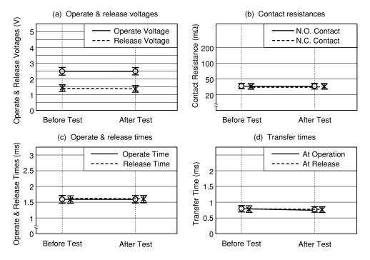
Figure 5.3 (1) Moisture Resistance Test
