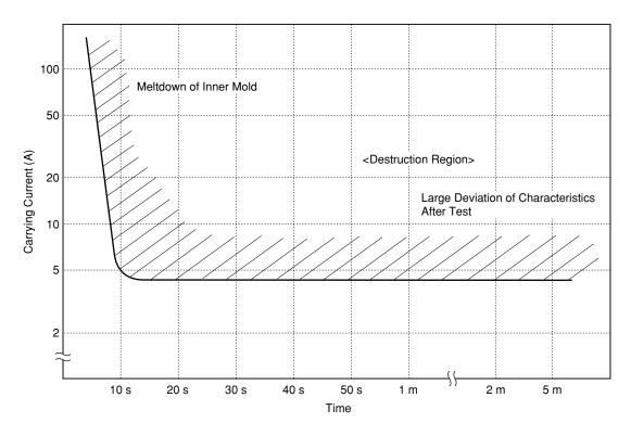
Figure 3.12 Resistance to Carrying Current
