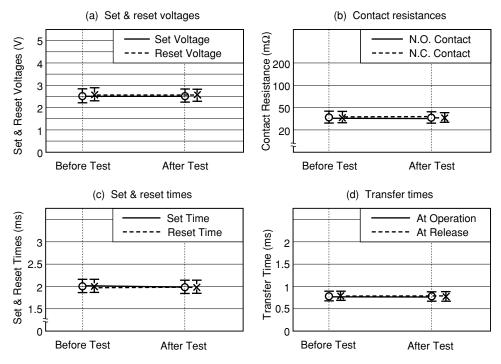
Figure 5.7 (2) Resistance to Solder Heat Test
