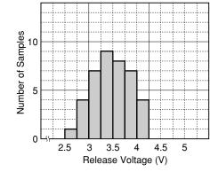
(3) Latching of single-wound coil, 5-V type (EC2-5S)
