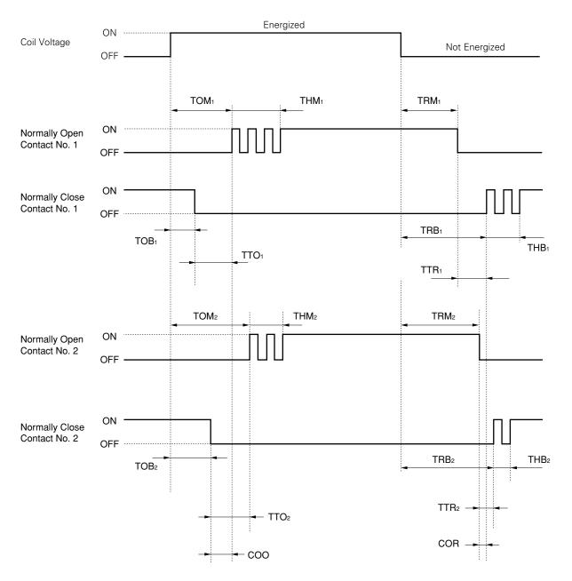
Figure 4.4A Timing Chart of Coil and Contacts
