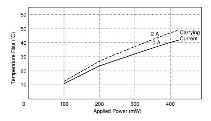
Figure 3.4 Coil Temperature Rise
