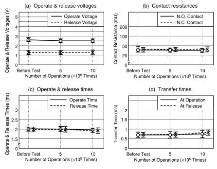
Figure 5.17 Inductive Load Test
