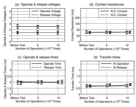
Figure 5.13 Resistive Load Test B
