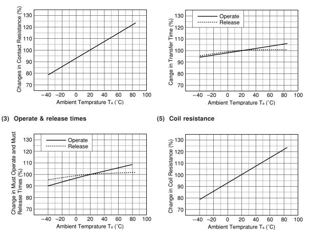
Figure 3.7 Temperature Characteristics
