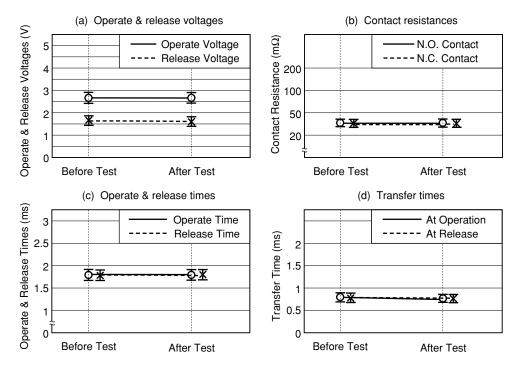
Figure 5.3 (3) Moisture Resistance Test
