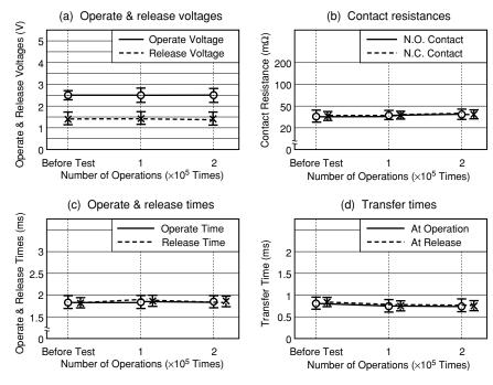
Figure 5.18 Resistive Load Test F
