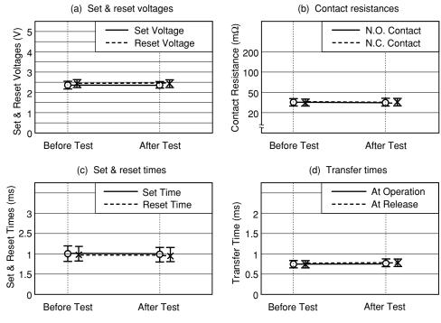
Figure 5.4 (2) Heat Shock Test
