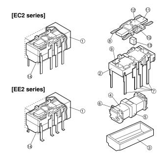
Figure 2.1 Structure of the EC2/EE2 Series Relay
