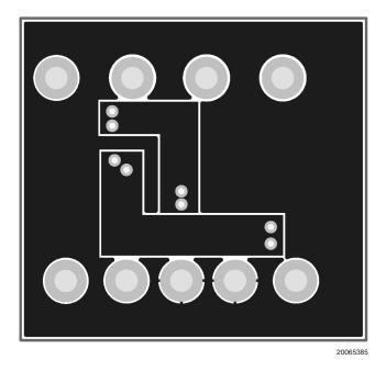
FIGURE 4. Evaluation Board Layout (2X Magnification)
