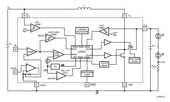
FIGURE 2. LM3501 Block Diagram
