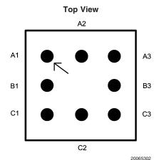
8-bump micro SMD  $T_{J(MAX)} = 125^{\circ}C$ ,  $\theta_{JA} = 220^{\circ}C/W$  (Note 3)
