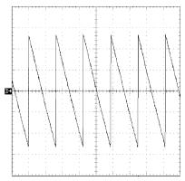
$V_{OUT}$  open circuit and equals approx. 15V DC,  $V_{IN}$  = 3.0V 3)  $V_{OUT}$ , 200mV/div, AC
