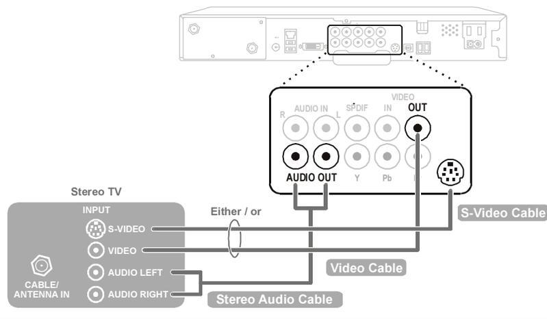
*This video connection method doesn't support High Definition video. For more information, see "Connecting your DCT6200 to an HDTV" on page 9.*
