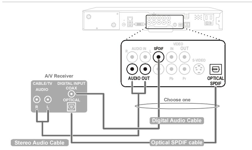
After you have finished connecting your DCT6200, see “Setting Up Your New DCT6200 for Digital Cable Services” on page 22.
