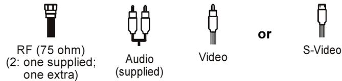
The cable configuration described here may be used for a mono or stereo VCR, because the VCR audio and video jacks are not used.
