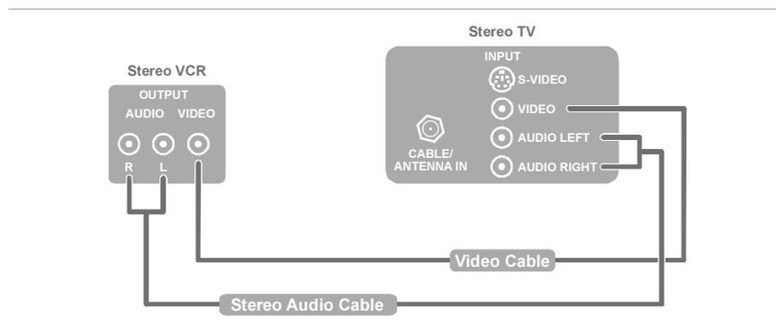
*This video connection method doesn't support high definition video. For more information, see "Connecting your DCT6200 to an HDTV" on page 9.*
