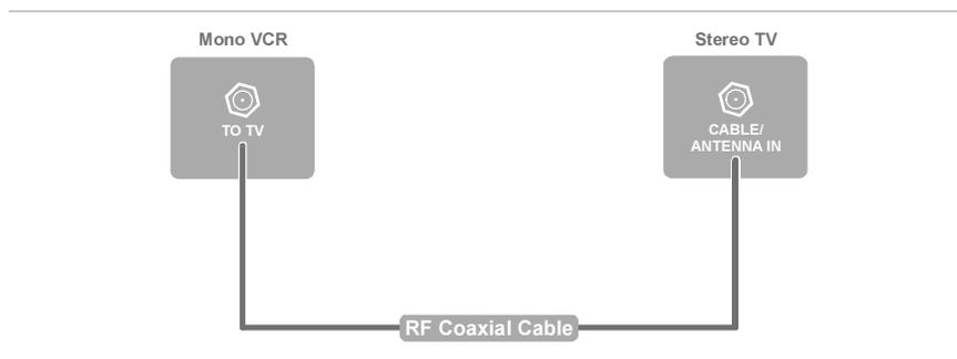
*This video connection method doesn't support high definition video. For more information, see "Connecting your DCT6200 to an HDTV" on page 9.*
