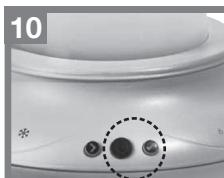
④-Button blinks green when the warming cycle is completed (Temperature of 34 °C +/- 3 °C is achieved).
