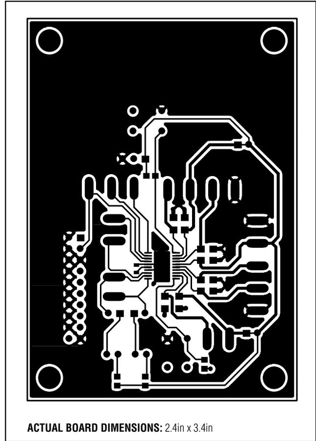
Figure 4. MAX1799 EV Kit PCB Layout—Component Side
