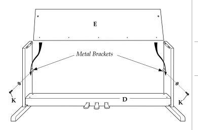
While lifting the piano keyboard unit on both ends (one person on each side), carefully lower it and slide the guide screws all the way forward into the brackets at the top of the piano stand (see the illustration in Step 11 for details).
