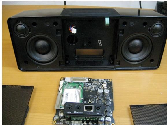
Figure 4: Main board removed, exposing the rear of the main board and acoustical chamber.
