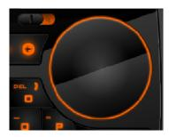
In touch-pad mode, the ClickPad functions like a touch pad. Onscreen cursor navigation is done by moving a finger across the ClickPad, which is perfect for Web surfing or other traditional computer operations. Note the orange backlighted ring around the ClickPad.
