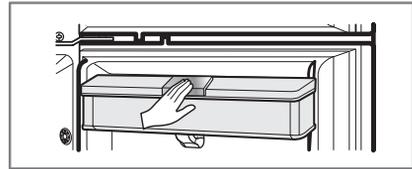
3. The water tank is optional removable part which can be applied to enlarge the storage capacity. You can use the upper basket after removing the water tank and closing up the hole with a plug. The plug is enclosed with the egg tray.
