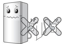
Prevent the power cord from being squeezed or imprinted if the refrigerator is pushed in after the power plug is extracted during the installation.
