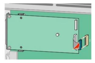
**12** If a printer hard disk was previously installed, then attach the printer hard disk to the ISP. For more information, see "Installing a printer hard disk" on page 30.
