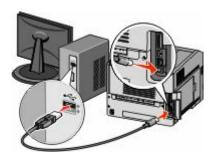
**Note:** After the printer is configured, the software will instruct you to disconnect the temporary USB cable so you can print wirelessly.
