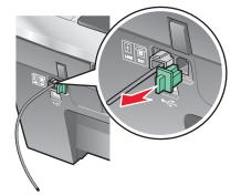
4 Connect the other telephone cord to a telephone, and then plug it into the EXT port is of the printer.
