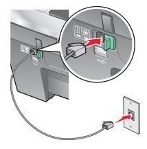
**3** Remove the protective plug from the EXT port  $\stackrel{\frown}{\boxplus}$  of the printer.
