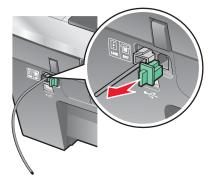
**4** Connect a second telephone cord from the telephone to the computer modem.
