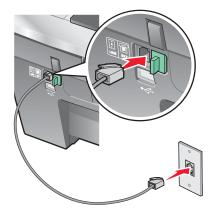
**3** Remove the protective plug from the EXT port  $\stackrel{\text{(iii)}}{=}$  of the printer.
