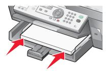
4 Adjust the paper guides to rest against the left, right, and bottom edges of the paper.
