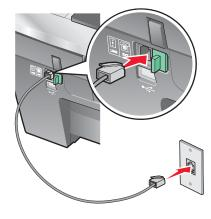
**3** Remove the protective plug from the EXT port III of the printer.
