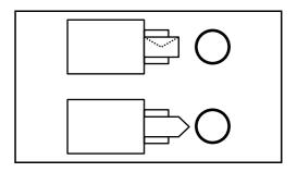
**IMPORTANT:** How to load envelope (orientation and facing) will differ depending on the type of envelope. Be sure to load it in a correct way. Otherwise printing may be done in wrong direction or on wrong face.
