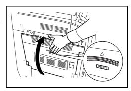
**16** Open the Multi Purpose Tray and remove the filters F1 and F2.
