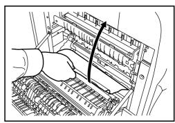
**3** Lift duplex unit and remove the jammed paper.
