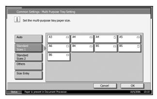
If you have chosen [Size Entry], press [+] or [–] to enter X (horizontal) and Y (vertical) sizes. You may enter the size directly using the numeric keys by pressing [# Keys].
