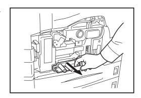
Open paper feed unit cover (A3) and remove the jammed paper.
