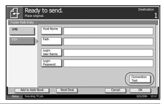
**NOTE:** *Connected.* appears when connection to the destination is correctly established. If *Cannot connect.* appears, review the entry.
