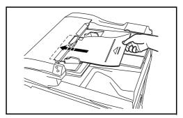
**CAUTION:** Confirm that the original width guides exactly fit the originals. If there is a gap, readjust the original width guides. The gap may cause the originals to jam.
