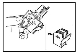
Insert the staple case fully to the end. Pull to remove the paper tape wound on the staple case.
