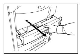
2 Holding the paper width adjusting tab, move the paper width guide to fit the paper.
