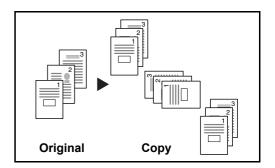
**NOTE:** To use offset function, load the same sized paper with different orientation in the paper source other than the selected paper source. The paper sizes supported in Offset are A4, B5, Letter and 16K.
