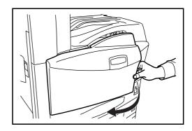
Push up the toner container stopper and slowly pull out the used toner container until its handle is visible.
