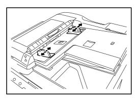
Place the originals. Put the side to be scanned (or the first side of two-sided originals) face-up. Slide the leading edge into the document processor as far as it will go. The originals placement indicator will be lit.
