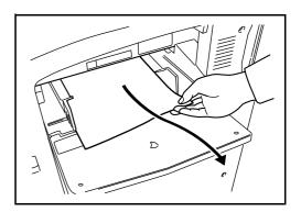
2 If a paper is jammed inside, lift the lever to remove the paper.
