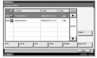
**NOTE:** To cancel the selection, press the check box to remove the check mark.
