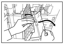
If the paper is torn, pull paper feed unit (A2) all the way out and lift it slightly to remove the paper.
