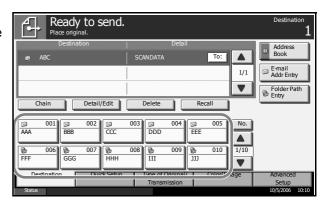
**NOTE:** If the **one-touch** key for desired destination is hidden on the touch panel, press  $[\ \ \ ]$  or  $[\ \ \ ]$  to scroll and view next or previous **one-touch** key.
