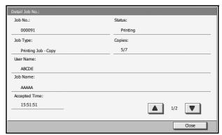
**NOTE:** Press [▲] or [▼] to view next detail. In the sending job, view the destination by pressing [Detail] of *Destination* or *Status/Destination*.
