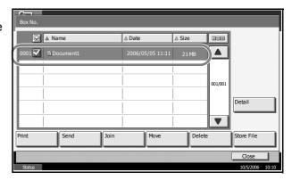
**NOTE:** Multiple documents cannot be selected and printed. To cancel the selection, press the check box to remove the check mark.
