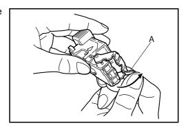
Clear the staple jammed in the cartridge end (staple-loaded side).
