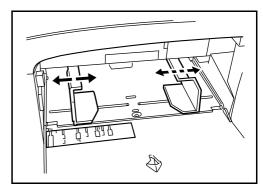
In the case of the landscape form envelope, close the flap. Insert the envelope all the way along the width guides, keeping the printing side face-up and with the flap positioned backward.
