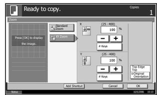
(horizontal) and Y (vertical). You can also enter the magnification directly using the numeric keys by pressing [# Keys].
