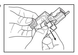
4 Holding the staple holder in your left hand and a new staple case in your right hand, insert the staple case into the staple holder in the direction of an arrow.
