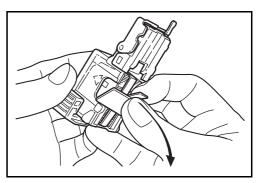
Insert the staple holder into the slot of the staple unit again.
