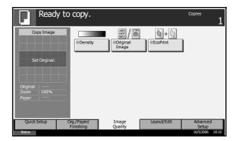
Adjust density manually pressing [-3] (Lighter) to [+3] (Darker). You can change the density level [-3] (Lighter) to [+3] (Darker) by half a step.
