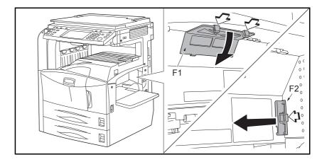
17 Clean the filters using a vacuum cleaner or the like.
