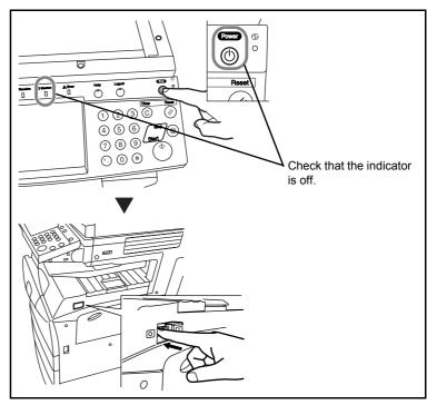
**2** Connect a LAN cable to the network interface located on right side of the body.
