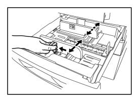
3 Using the paper length adjusting tab, move the plate to fit the paper.
