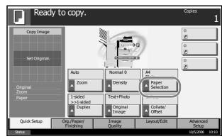
**NOTE:** Select paper size manually, if necessary, instead of using automatic paper selection.
