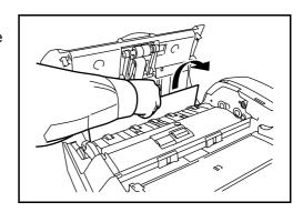
If it is difficult to remove the original, turn the feed dial. The original will be pushed to a place where it is easier to remove.
