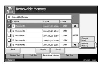
**4** Remove the USB memory after *Removable Memory can be safely removed* is displayed.
