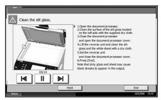
**IMPORTANT:** Lightly wipe the slit glass with a dry cloth. To remove adhesive material or ink, apply alcohol to a cloth and wipe lightly. Do not use water, thinner, or organic solvents.
