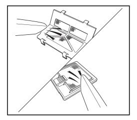
**CAUTION:** Do not wash the filters with water. Do not use the attached cleaning brush.
