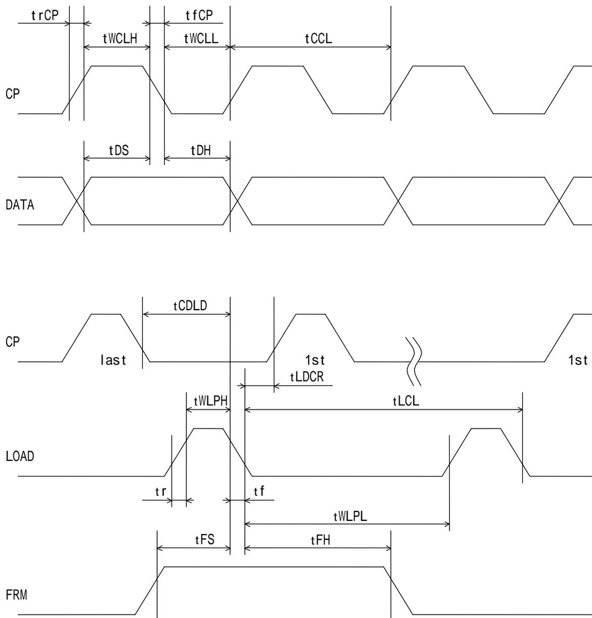
11-1. Switching characteristics ( $V_{DD} = 5.0V$ )
