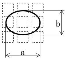
$d = (a + b) / 2$ <table border="1" data-bbox="606 1579 1412 1848"> <thead> <tr> <th>Category</th> <th>Size (mm)</th> <th>Acceptable number</th> </tr> </thead> <tbody> <tr> <td>A</td> <td>d ≤ 0.2</td> <td>Neglected</td> </tr> <tr> <td>B</td> <td>0.2 &lt; d ≤ 0.3</td> <td>5</td> </tr> <tr> <td>C</td> <td>0.3 &lt; d ≤ 0.5</td> <td>3</td> </tr> <tr> <td>D</td> <td>0.5 &lt; d</td> <td>0</td> </tr> </tbody> </table> | Category
