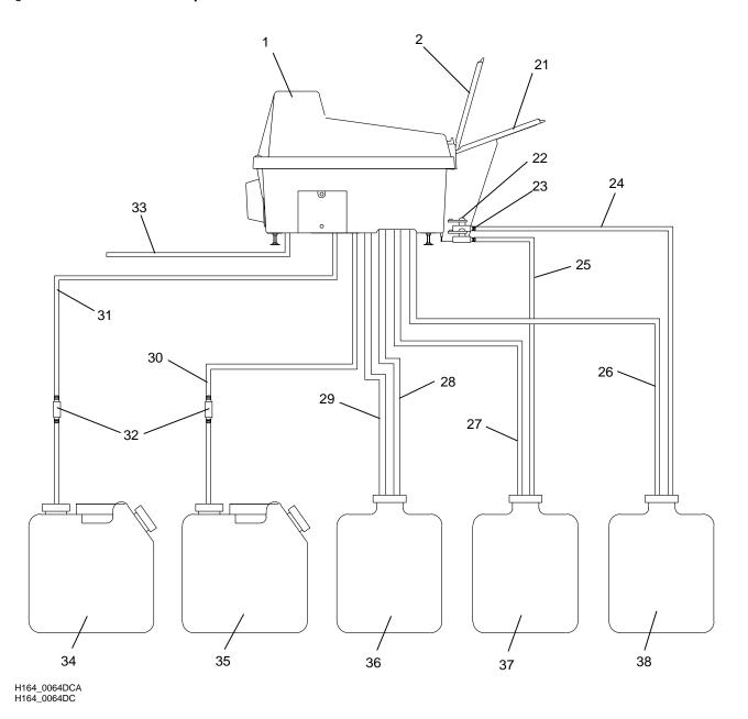
Item No. Description Item No. Description 26 **Developer Overflow Hose** 35 Developer Replenishment Container 27 Fixer Overflow Hose 36 Wash Water Drain Container Wash Water Drain Hose 28 37 Fixer Drain Container 29 Wash Water Overflow Hose 38 **Developer Drain Container** 30 Developer Replenishment Hose 39 **Developer Tank** 31 Fixer Replenishment Hose 40 Fixer Tank Wash Tank 32 Replenishment Filter 41 33 Screen Filter Wash Water Supply 42 34 Fixer Replenishment Container 43 Pitcher
