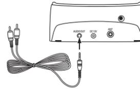
2. Plug the audio cable's white (L ch.) and red (R ch.) connectors into your audio system's available audio input.
