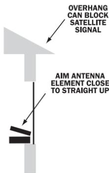
Use this map as a general placement guideline—some experimentation may be needed to obtain the best reception in your particular situation. See pg. 27, Antenna Aiming, for more information about using the ANTENNA SIGNAL screen to aim the antenna.
