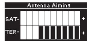
Moving the antenna location may adjust the bar graph signal strength indications and insure optimum reception. Pressing the Control Knob, the menu button, or the remote Select button returns to the top level Menu Options.
