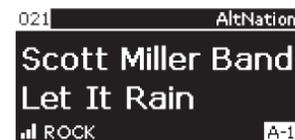
Use the Control Knob (or the remote CH buttons) to move through the Presets. Each time you change a Preset, its number will appear on the display and the channel will play.
