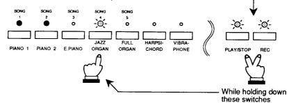
To cancel deletion, press the SONG switch again so that the LED lights before releasing the PLAY/STOP and REC switches.
