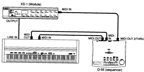
When connected as shown in the illustration, you can record songs played on the digital piano with a sequencer, and play them back as many times as you like. This is very useful for practice. You can also play back the contents of the digital piano recorder and record them with the sequencer.
