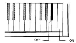
White key (ON): The piano will output sound when the keys are struck. Black key (OFF): Sound will be output only when MIDI data is received, and not when the keyboard is played.
