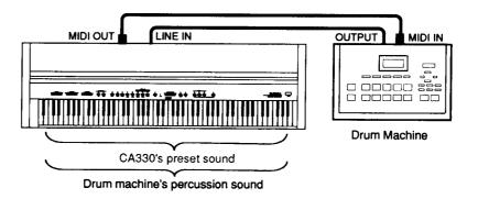
When connected as shown in the illustration, you can not only play along with the rhythm from the drum machine, you can also play the drum machine by striking the keys on the digital piano.
