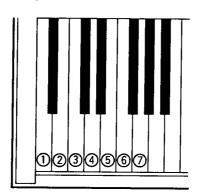
Volume is set to its lowest with the "1" key and at its highest with the "7" key. The "4" key is the factory setting.
