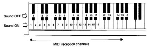
Use the 16 white keys at the left end of the keyboard to set the channels to ON. Use the 16 black keys at the left end of the keyboard to set the channels to OFF.
