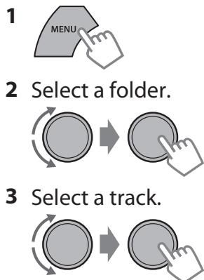
If the USB device contains many folders or tracks, you can fast search for desired folder or track by turning the control dial quickly, or use Quick Search. (☞ page 11)
