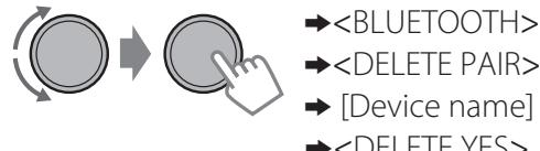
"DELETED" appears when the device is deleted.
