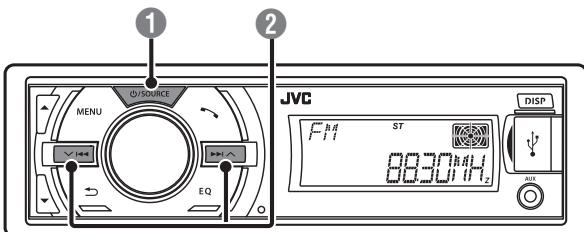
"ST" lights up when receiving an FM stereo broadcast with sufficient signal strength.
