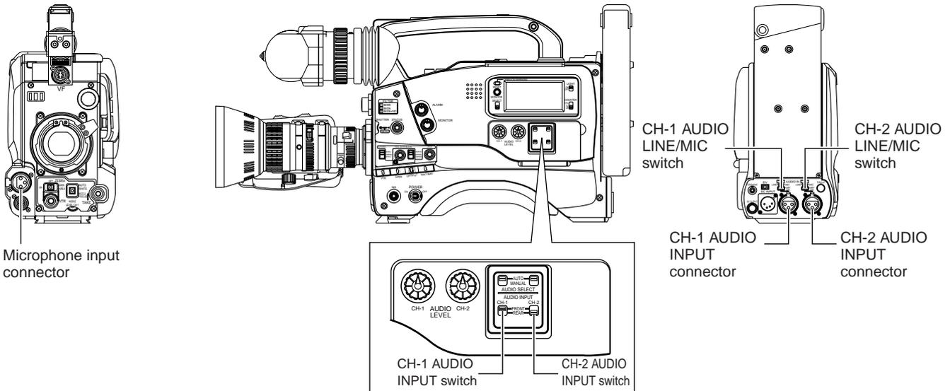
The GY-DV500 is provided with the microphone connector on the front section and the two AUDIO INPUT connectors at the rear section for audio input.
