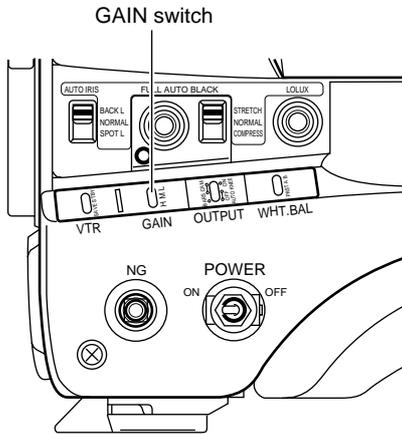
This switch allows the gain to be boosted when the illumination of the subject is insufficient.
