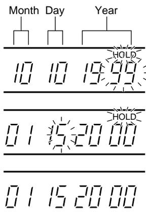
1. Turn ON the power and set the counter display to the date/time mode.
