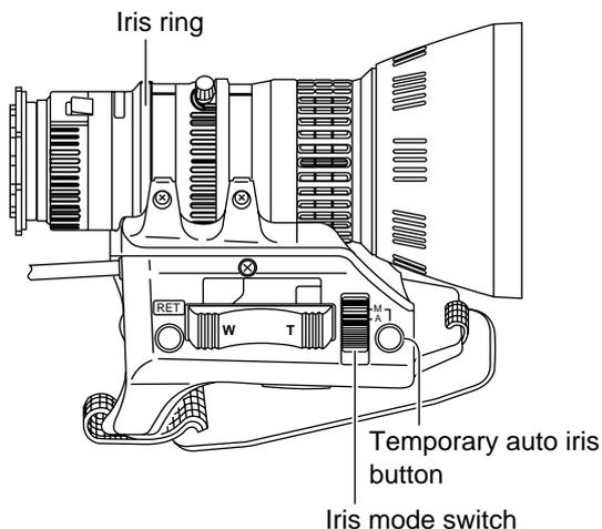
The lens iris can be adjusted using any of the following three methods.
