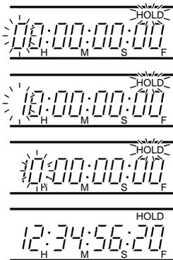
1. Display the time code on the counter display. Set the COUNTER switch to "TC".
