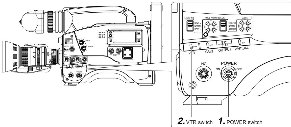
1. Turn the POWER switch to ON.
