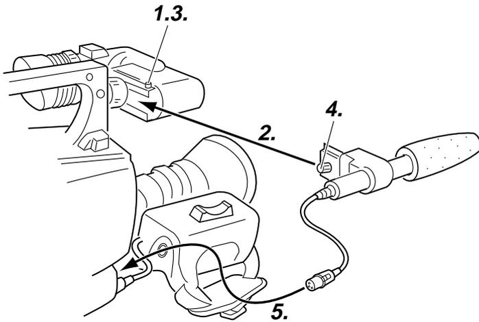
Connecting the provided microphone to the viewfinder. The provided microphone is a phantom microphone.
