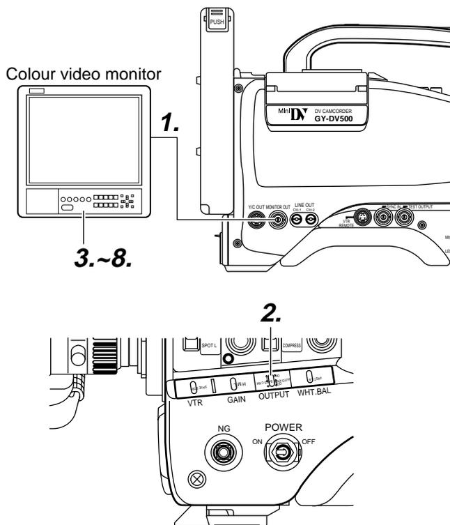
Display the camera built-in color bar signal on the video monitor and adjust the colors, contrast and brightness.
