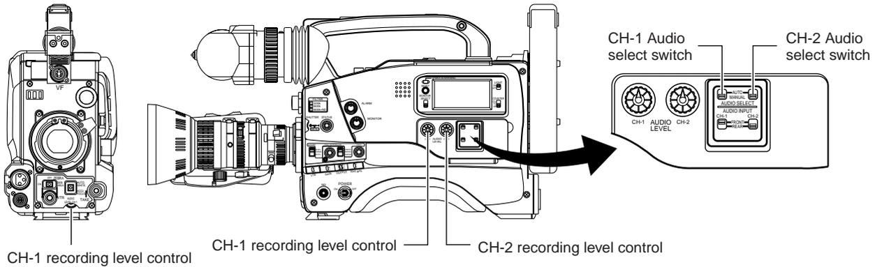
For each audio channel, use the AUDIO SELECT switches to select whether the recording level adjustment should be set to AUTO mode or MANUAL mode.
