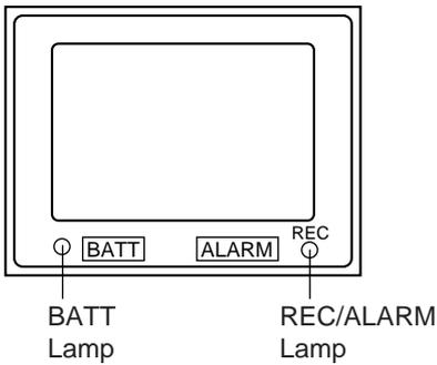
The viewfinder has two LED indicators below the screen. These LEDs light or blink to indicate the present status of the camera or the VCR.
