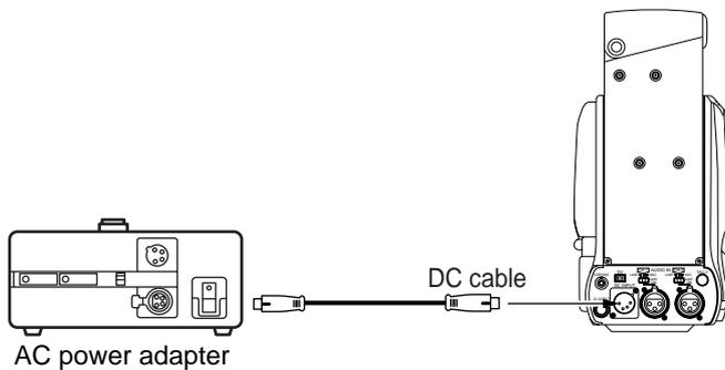
Do not use any power source with large fluctuations in the power source voltage, or power sources generating noise, such as ripples.
