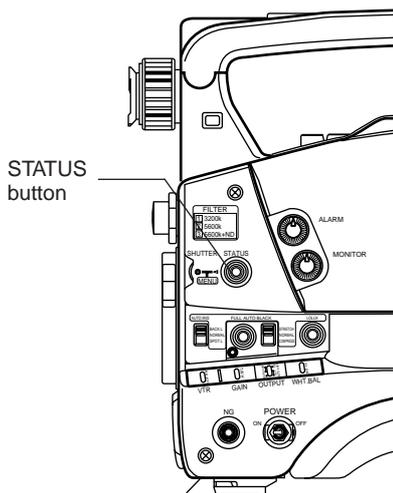
Press the STATUS button during normal screen display to show one of the status screens in the viewfinder. One of the three status screens will be displayed every time the button is pressed.
