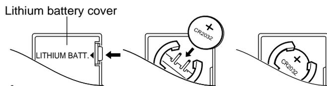
1. Push the lithium battery cover in the direction of the arrow as illustrated and remove the cover.
