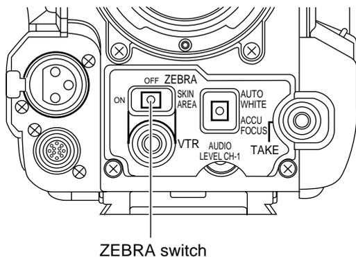
By setting the ZEBRA switch to **ON**, oblique stripes (zebra pattern) can be displayed in the sections with a luminance level of 70% to 80% or sections with levels over 100% in the viewfinder.
