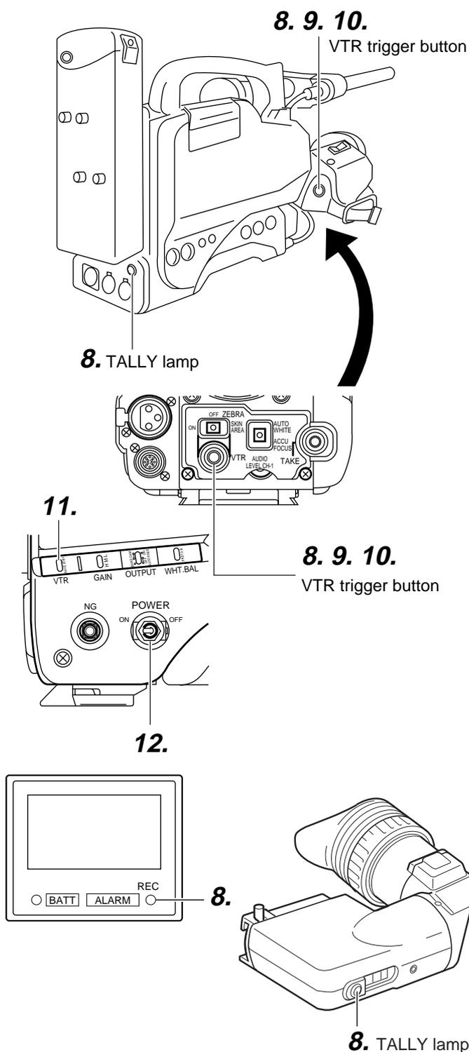
**8.** Press the VTR trigger button on the GY-DV500 or lens to start recording.
