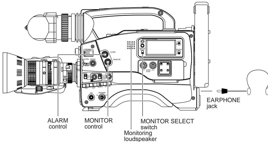
The audio input during recording, in record-pause or stop mode can be monitored through the monitoring loudspeaker or earphone.
