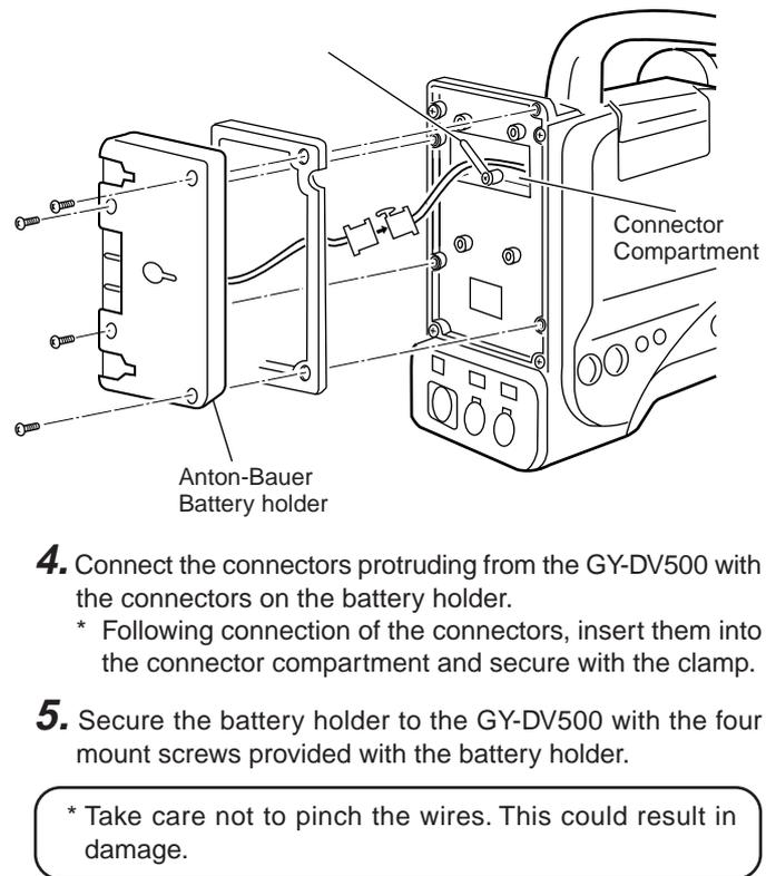
**Attaching and Detaching an Anton-Bauer Battery Pack**
