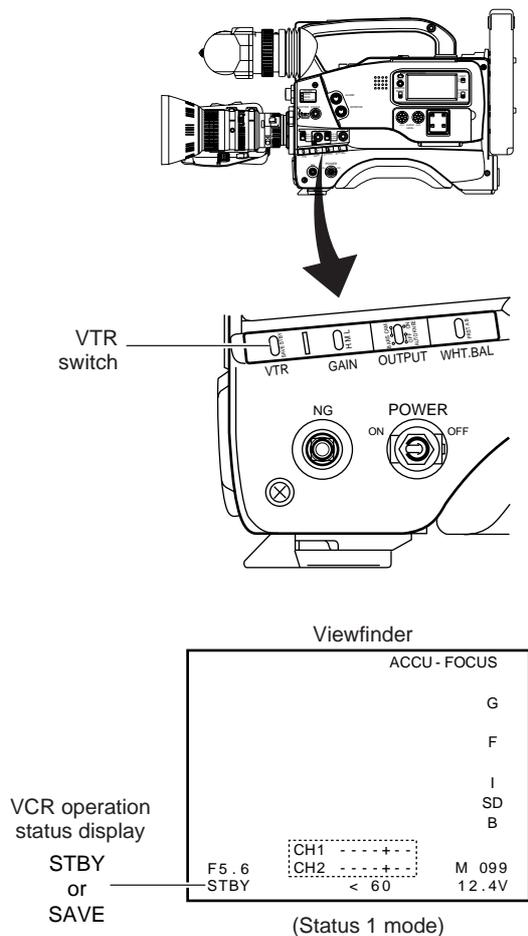
When a recordable videocassette is loaded, the GY-DV500 enters the record-pause mode. However, the record-pause operation condition differs depending on the setting of the VTR switch.
