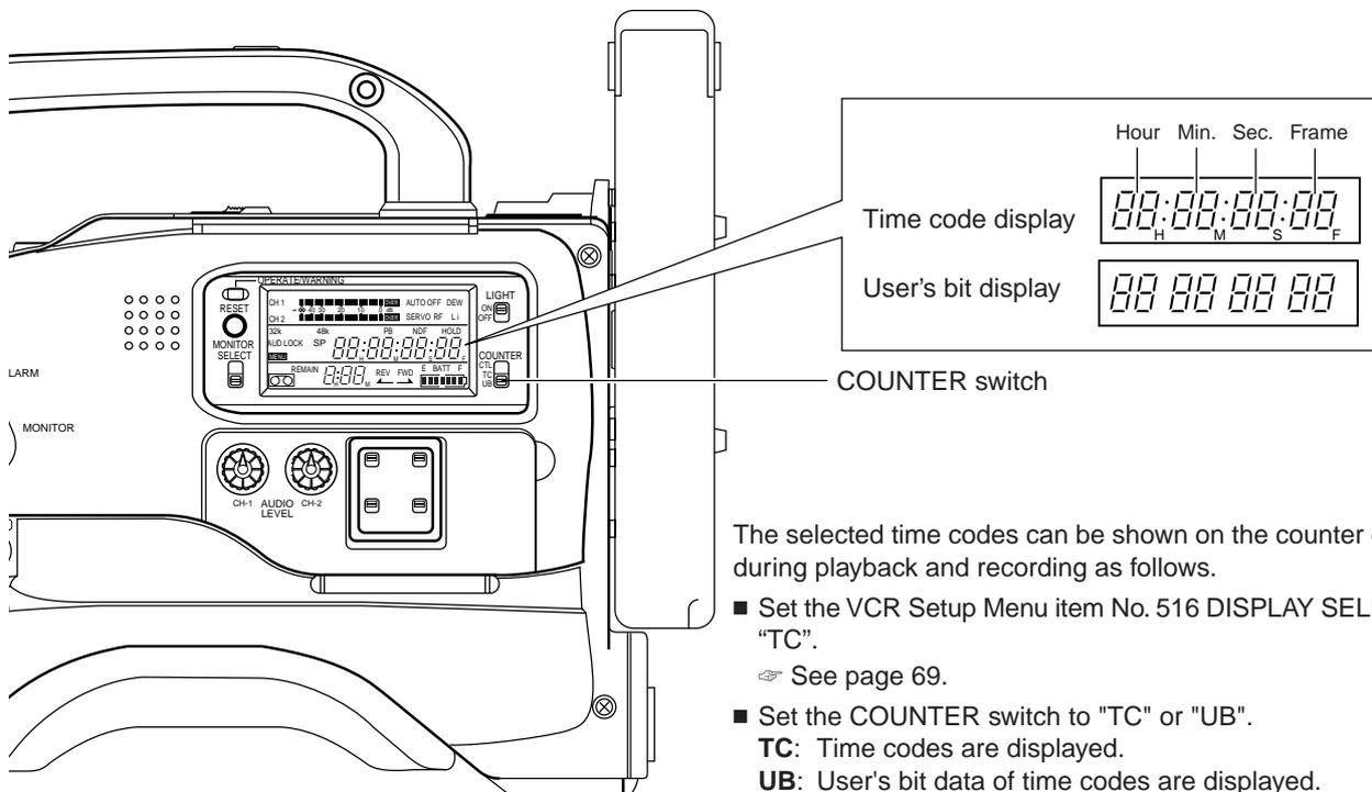
The selected time codes can be shown on the counter display during playback and recording as follows.
