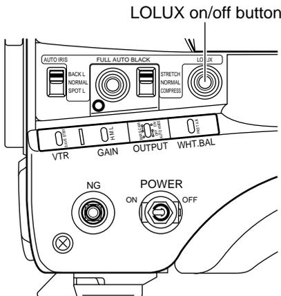
The LOLUX button is used when the illumination is still insufficient after compensating with the GAIN switch. Press the button to enter the LOLUX mode in which the gain is boosted by about 33 dB.
