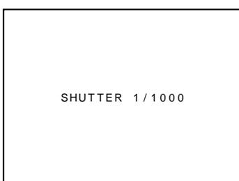
When the SHUTTER dial is pressed, a shutter speed is displayed (for approx. 5 sec.).
