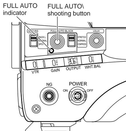
The FAS function provides a wide range of compatibility with shooting conditions that varies as you move between indoors and outdoors or between bright and dark locations. It eliminates the need to change the switch and filter positions every time you move.
