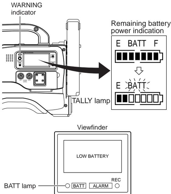
To display the remaining battery power accurately, set the VCR Setup Menu item No. 396 BATTERY TYPE according to the type of the battery pack in use.
