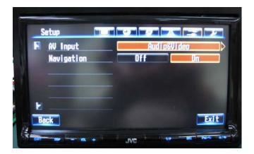
2) Once Navigation option as "ON" as shown above, Press "Disp" option then SatGuide application will launch in the device as shown below.
