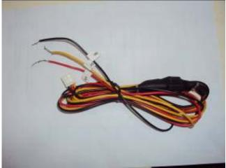
2) Connect the **RGB&Data cable** and **power cable** to GPS blackbox
