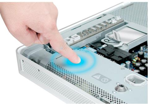
2. Locate the memory module(s) in the bottom right corner.
