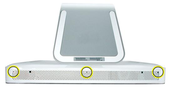
6. Holding the back cover by the metal foot, tilt the cover up. Lift the cover off the computer. Set the back cover aside.
