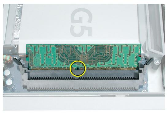
3. Press firmly on the memory module until it clicks into place. Use your thumb and index finger to push the module into the slot.
