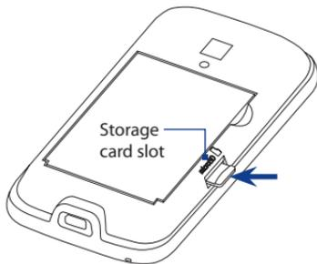
**Note** To remove the microSD card, press it to eject it from the slot.
