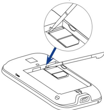
3. Slide the SIM card out from the slot with your other thumb or finger.
