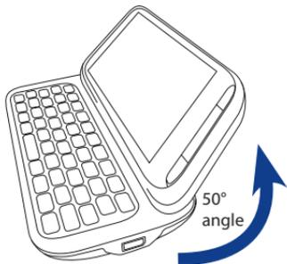
The maximum tilting angle of the screen is 50 degrees. Do not force the screen to tilt further than the maximum tilting angle as it will break the device.
