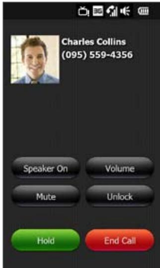
Tap the onscreen buttons to turn the speakerphone on, hold the call, change the in-call volume, and so on.
