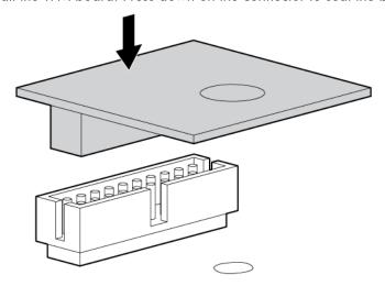
Install the TPM security rivet by pressing the rivet firmly into the system board.
