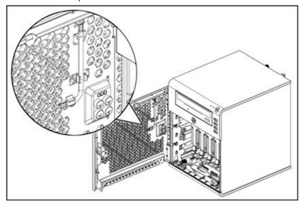
In performing hardware configuration, you must have the system screwdriver secured to the front panel door. All hardware screws used in the server can be removed or tightened by using the system screwdriver. All spare screws are located on the back side of the front panel door.
